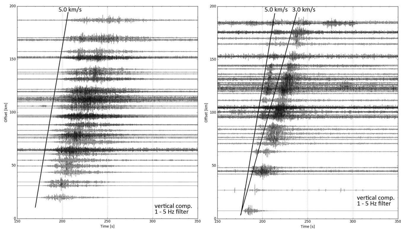
**Figure 3.** Record sections (signal vs. distance) of the vertical component for two large rockslides. All data are bandpass-filtered between 1 and 5 Hz. Left: Kleine Gaisl, Italy, 2016-08-19, as an event example that does not show a clear second arrival. Right: Mellental, Austria, 2016-03-25, which does show a distinct second arrival for stations farther than 50 km from the origin. Black lines mark expected arrival times for a constant travel-time of 5.0 km/s and 3.0 km/s, respectively.
