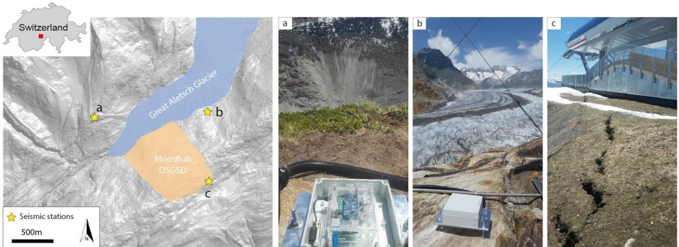
**Figure 1: (left) Map of the area of investigation with indication of the location of the three RS seismic station installed starting from May 2017. (a-c) Pictures of the RS installation (a, RS-1; b, RS-2; c, RS-3). Continuous records of seismic signals on the 3 stations are available since beginning of July 2017.**
