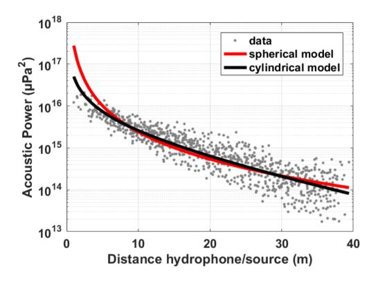
Figure 5: Data from the Leysse river. Measured acoustic power ( $\mu Pa^2$ ) in function of the distance between the hydrophone and the active source. Results obtained in the third-Octave band centered on 1 kHz. Spherical and cylindrical fits are in thick lines.
