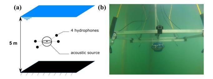
Figure 1: (a) schematic design of the test characterizing the system of emission; (b) photography of the immerged system in the lake of the Bourget (France).
