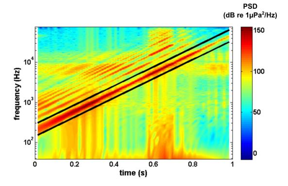
Figure 4: Short-term spectrogram of a chirp monitored by a hydrophone in the Leysse River. The black lines indicate the octave band centered around the instantaneous frequency of the theoretical logarithmic chirp.
