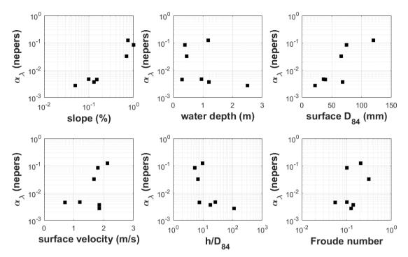
Figure 10: representation of the attenuation coefficient per wavelength ( $\alpha_{\lambda}$  in nepers) in function of river characteristics: (a) local slope (%); (b) average water depth (m); (c) surface  $D_{84}$  (mm) of the closest emerged bars; (d) average surface velocity (m/s); (e) ratio of water depth (m) over surface  $D_{84}$  (m); (f) Froude number computed with average flow velocity (m/s) and water depth (m).
