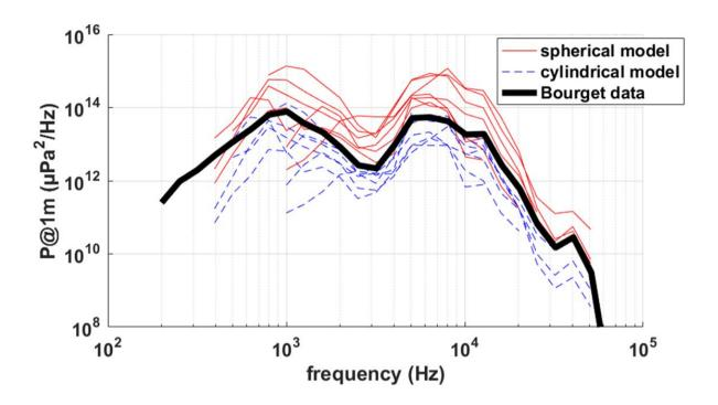
Figure 7: Power spectral density of the source power  $(P_{@1m}$  in  $\mu Pa^2/Hz)$  estimated with spherical and cylindrical models for all experiments made in rivers and measured in the Bourget lake.
