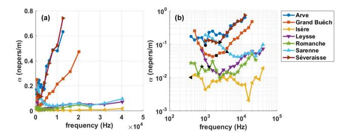
Figure 8: attenuation coefficient ( $\alpha$  in nepers/m) obtained when using a cylindrical model of the geometrical spreading loss: (a) linear and (b) logarithmic scales. Black symbols indicate the cutoff frequency computed with eq. (8), sound speeds of 1500 m/s and 1600 m/s in the water and sediment layer, respectively.
