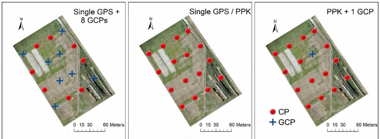
**Figure 3: Distribution of GCPs and CPs and illustration of the different georeferencing configurations: *Single GPS*, *Single GPS + 8 GCPs*, *PPK*, *PPK + 1 GCP*. Note: Cross validation was implemented in *PPK + 1 GCP* configuration, i.e., one single control point was used as GCP in each processing.**
