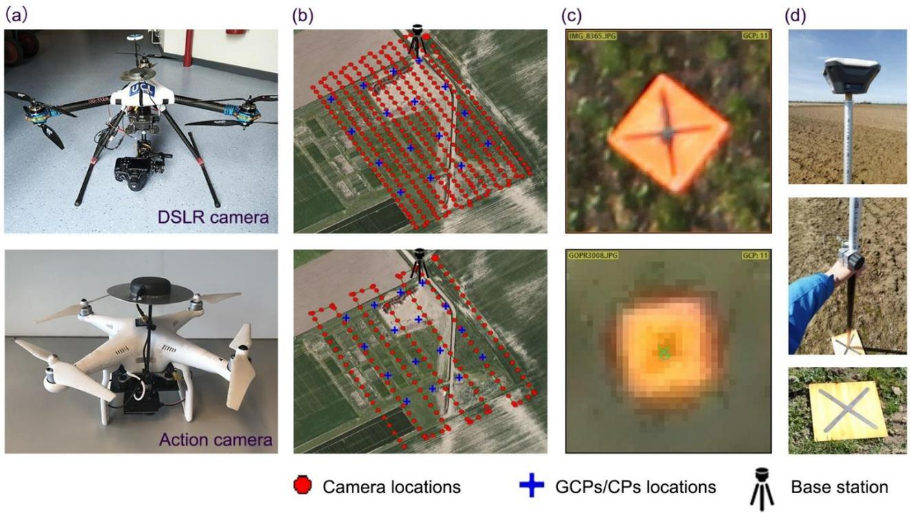
5 **Figure 2: Experimental setup:** (a) UAV/camera setup: DSLR camera (EOS 550D) mounted on RPAS Type Y6, Action camera (GoPro Hero 3) mounted on a Phantom 3 Advanced (b) Parallel flight lines (Top: RPAS Type Y6 with DSLR camera; Bottom: Phantom 3 with action camera) and GCPs/CPs distribution (c) How GCPs/CPs displayed in the images and (d) Measurement of GCPs/CPs.
