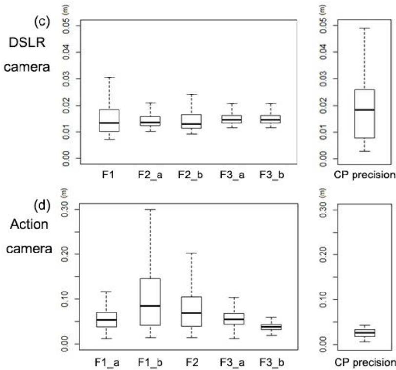
Figure 5: Precision maps derived from Monte Carlo simulation. (a) MC map of DSLR camera, dataset: F3\_a (b) MC map of action camera, dataset: F2\_b (c) boxplots of MC precision of DSLR surveys (area of interest) (d) boxplots of MC precision of action camera surveys (area of interest)
