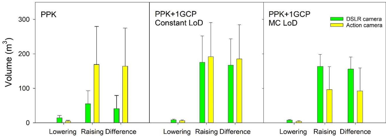
5 **Figure 6: Change detection based on DoD (datasets: F2, F3\_a of DSLR and action camera surveys). (a) Surface change map (b) Height profiles sampled at identical location from the corresponding DSMs before and after plowing. Line graph shows height profiles along the sample transect (X-axis: position along the transect, Y-axis: surface height) (c) Volumetric sediment budget.**
