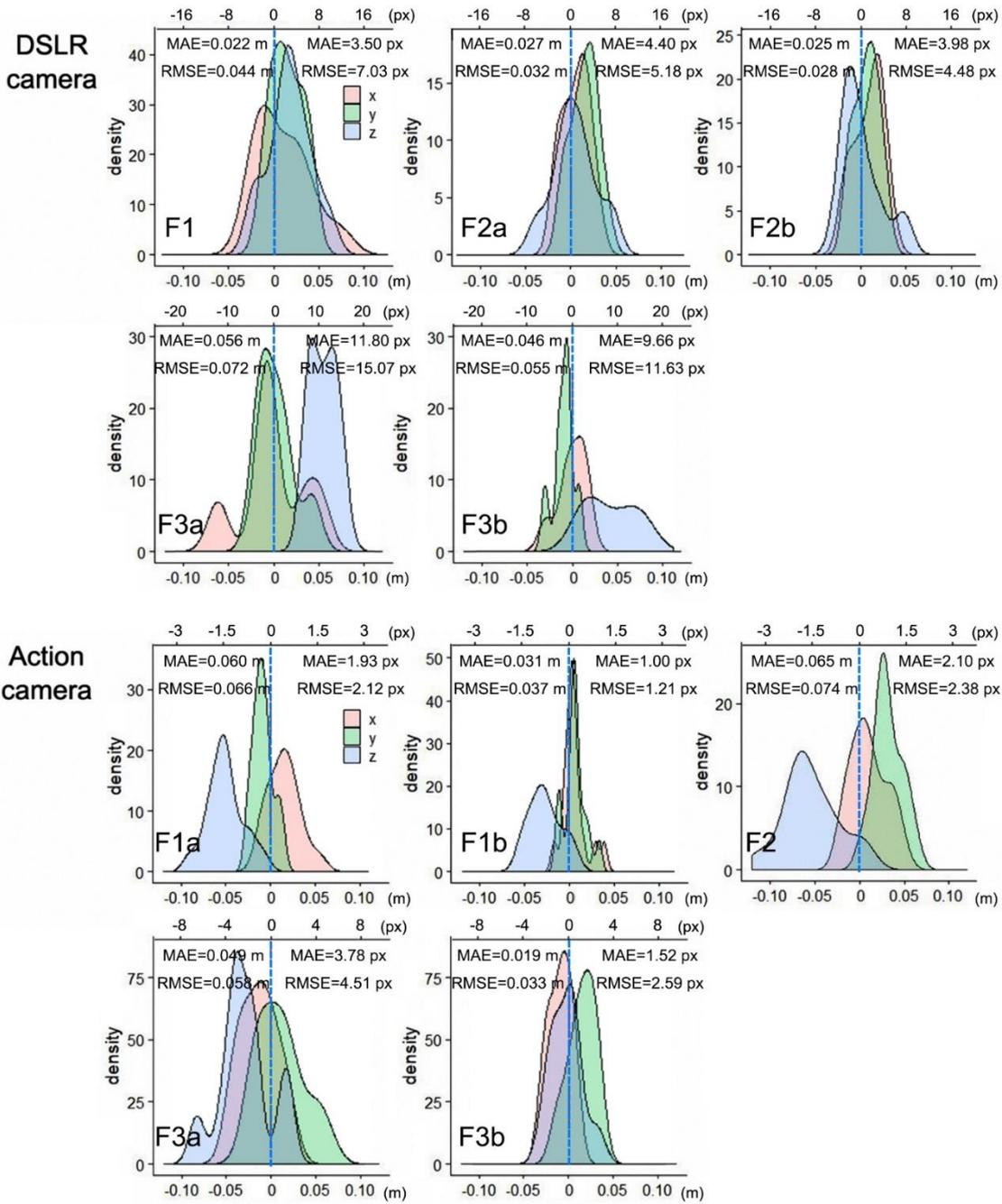
**Figure 4: Distribution of CP residuals on X, Y and Z directions of each survey. MAE and RMSE in legend indicate mean absolute error and root-mean-square-error of XYZ direction. Units are given in meters as well as pixels to standardise results in terms of the expected error incurred from the GSD at corresponding flight height.**
