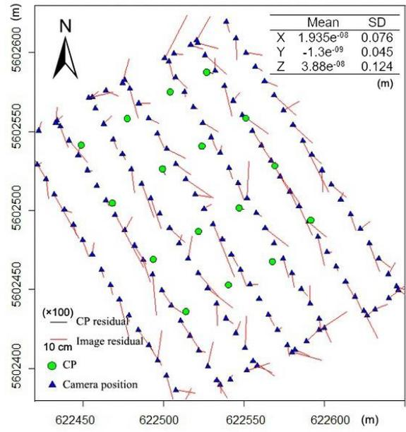
**Figure A2. Residuals on the images and CPs in planimetric view. Vectors give the horizontal residual component magnified by  $\times 500$  for DSLR survey (left) and  $\times 100$  for action camera survey(right). With inset mean value and standard deviation of the image residuals.**
