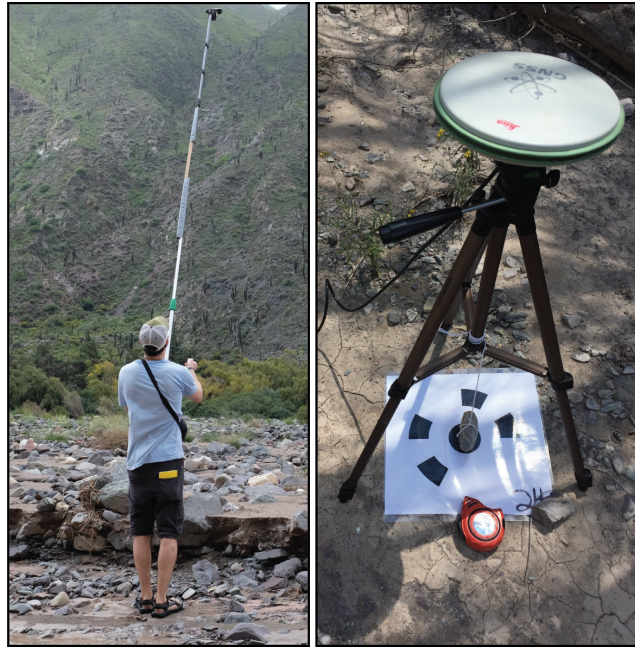
Figure 7. Sony \alpha 6000 24 MP-megapixel camera affixed to mast for photo collection at a height of 4.5–5 m (left) and differential GPS measurement of coded targets (right).
