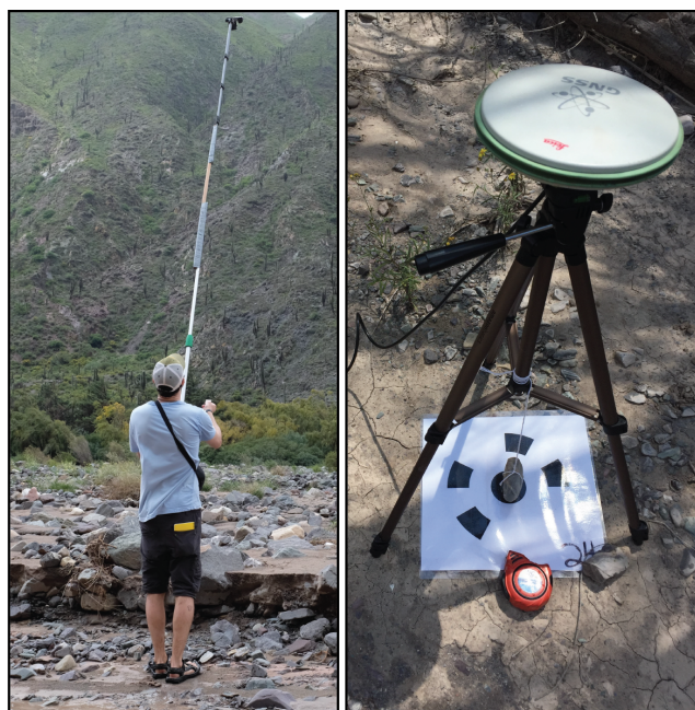
Figure 10. Sony \alpha 6000 24 MP camera affixed to mast for photo collection at a height of 4.5–5 m (left) and differential GPS measurement of coded targets (right).
