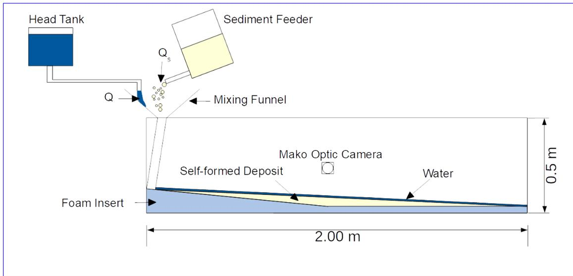
**Figure 1.** Simplified diagram of the experimental setup for the steep channel flume.
