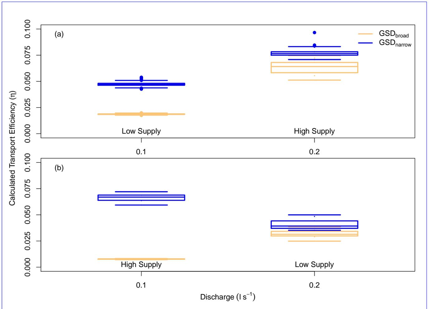
**Figure 8.** Distribution of transport efficiencies ( $\eta$  from  $\dots$ , calculated using Eq. (3). Plots separate experiments by relative sediment concentrations of (a) 1 and (b) for experiments 100L not 1 (i.e., 100H0.5 or 2). Text indicates sediment feed rate (low supply =  $1 \text{ g s}^{-1}$ , 200L and 200H high supply =  $2 \text{ g s}^{-1}$ ).
