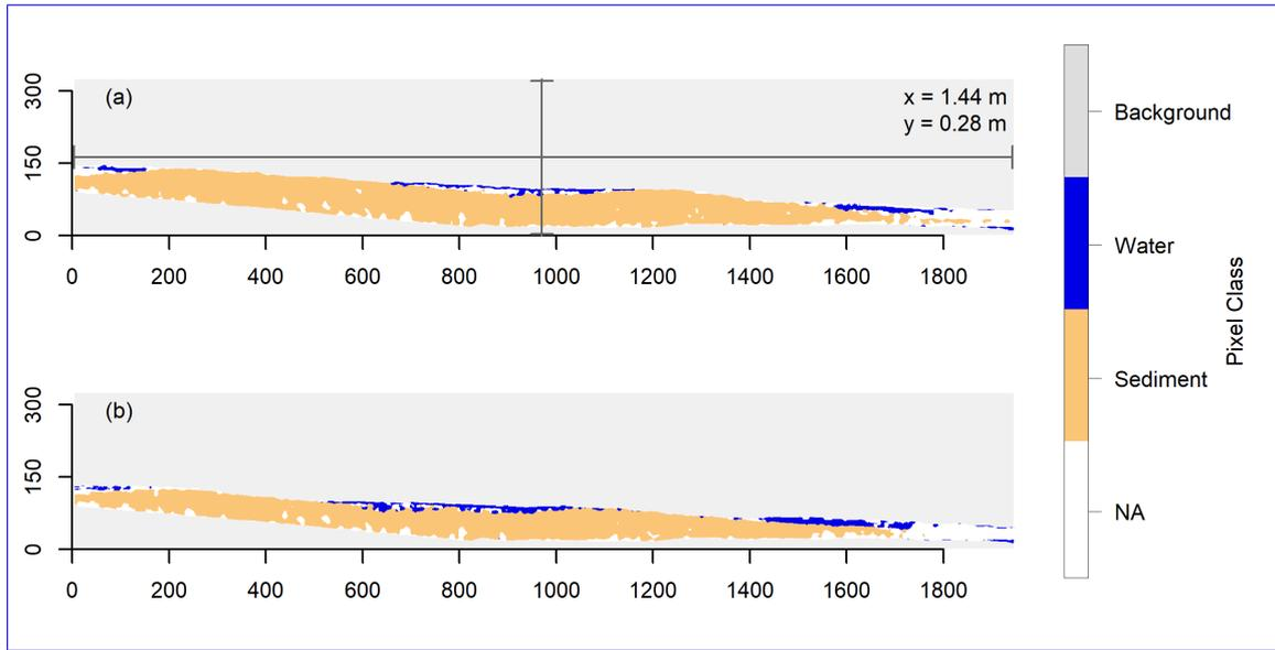
**Figure 4.** Output after image classification at end-the onset of aggradational-phases-output for Exp. 100L using (a)  $GSD_{T_{broad}}$  ( $T = 327-326$  min) and (b)  $GSD_{z_{narrow}}$  ( $T = 150-149$  min). Axes are pixel values of the raster, and real distances are provided for scale.
