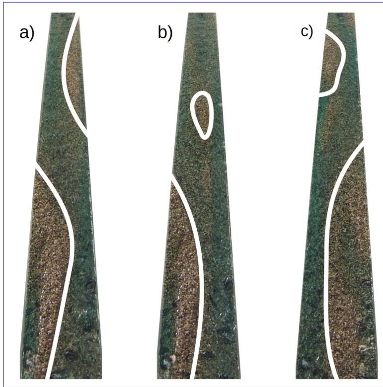
**Figure 10.** Three frames taken from the beginning, middle and end of a thalweg sweep event from the left side of the flume to the right and resulting in a switching of the thalweg position, in experiment 200H using GSD<sub>narrow</sub>. These frames correspond to approximately 28 s to 30 s of the accompanying video.
