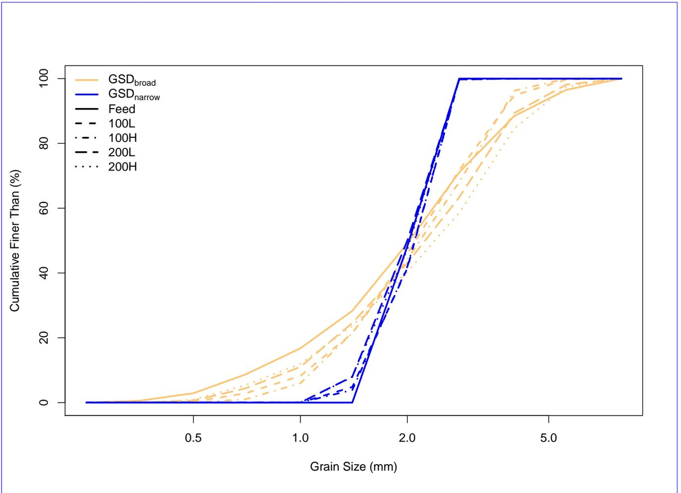
**Figure 7.** Size distributions of material output across the length of each experiment. Original grain size distributions are also provided.
