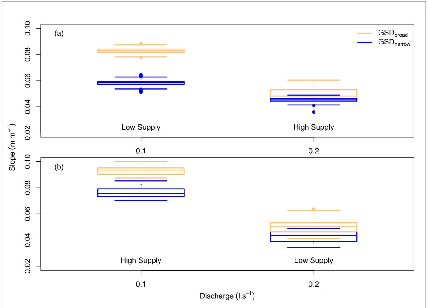
**Figure 6.** Distribution of slope values from the onset of transport onwards. Plots separate experiments by relative sediment concentrations of (a) normal (i.e., 1) and (b) not normal (i.e., 0.5 or 2) relative sediment concentration. Text indicates sediment feed rate (L low supply = 1 g s<sup>-1</sup>, H high supply = 2 g s<sup>-1</sup>).
