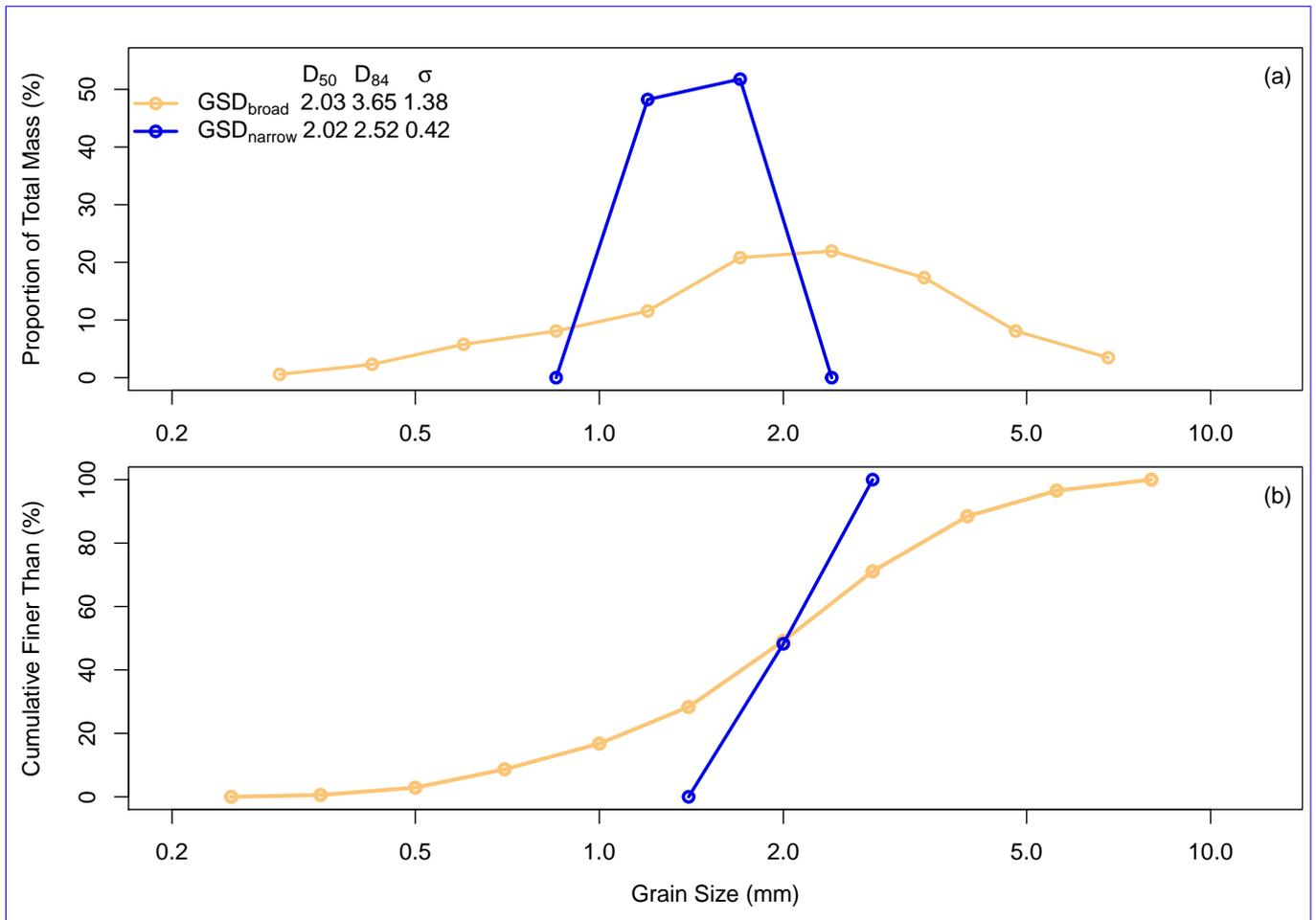
**Figure 2.** Grain size distributions for half-phi classes (a) individually and (b) cumulatively. Grain size metrics are shown in mm.
