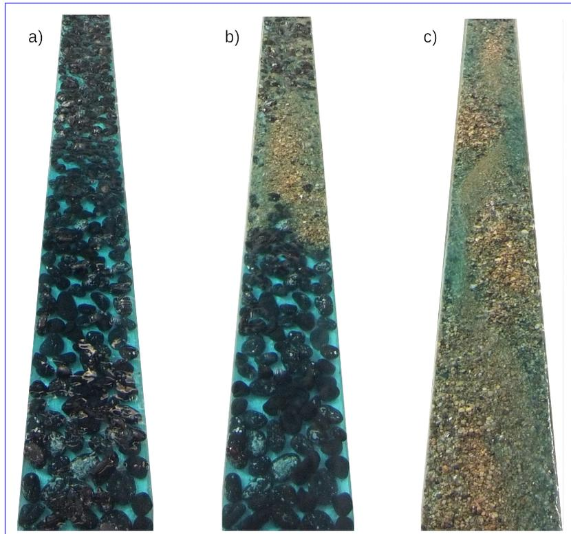
**Figure 3.** Example image-images of the black roughness element-sediment elements used to force subcritical flow, and their submergence taken during sediment output (a) beginning of experiment with full emergence, (b) partial submergence and (c) onset of transport, almost complete burial and submergence, from experiment G2Q100H200H using  $GSD_{broad}$ .
