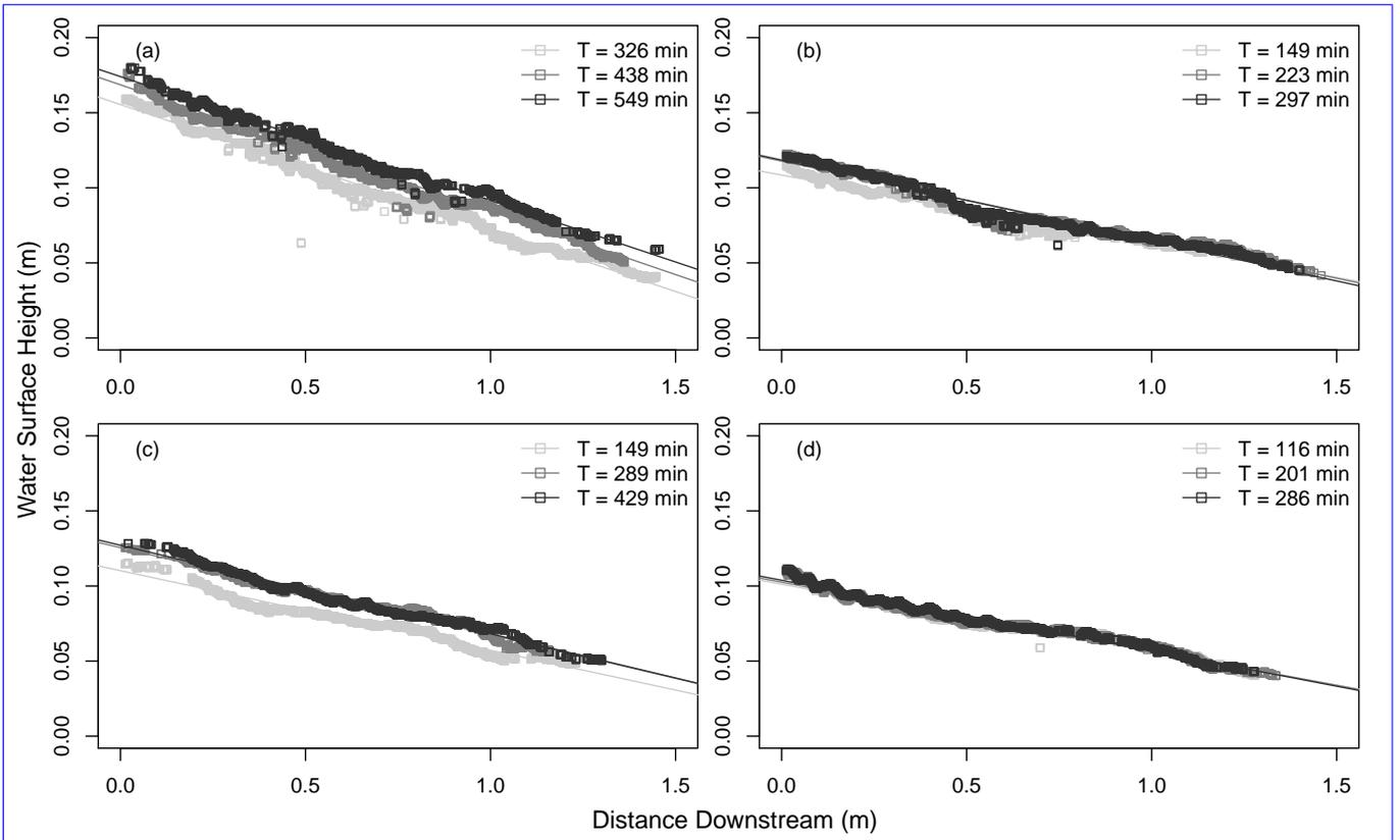
**Figure 5.** Example water surface profiles, and regressions used to derive slope, for experiments (a)  $GSD_{broad} 100L$ , (b)  $GSD_{broad} 200H$ , (c)  $GSD_{narrow} 100L$  and (d)  $GSD_{narrow} 200H$ . Times given in legend correlate to the onset of output, approximately halfway through the experiment, and the end of the experiment.
