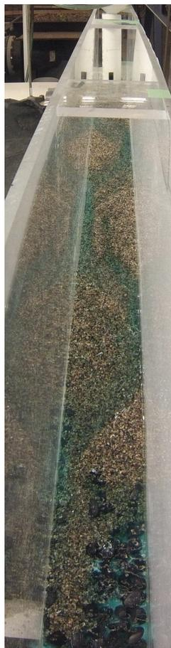
**Figure 3.** Example image of roughness element sediment submergence taken during sediment output, from experiment G2Q100H.
