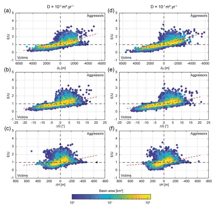
Figure 8: Effect of diffusivity. Note that the x axis is reversed for both Δχ and ΔH. Color scale indicates basin area. Red dashed lines correspond to the linear fits obtained for the reference model (see figure 6). (a) to (c) Same as Fig. 6d-f, with a diffusivity of 10<sup>-3</sup> m<sup>2</sup>.yr<sup>-1</sup>. (d) to (f) Same as Fig. 6d-f, with a diffusivity of 10<sup>-1</sup> m<sup>2</sup>.yr<sup>-1</sup>.
