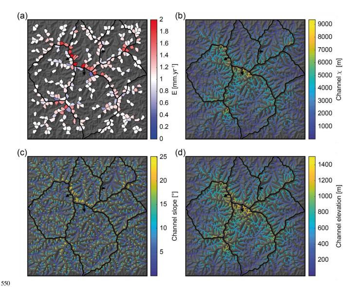
Figure 5: Denudation rates and cross-divide contrast metrics obtained for the reference model after 5 Myr. (a) Map of denudation rates for basins of 2-4 km<sup>2</sup>. Black thick lines correspond to basin divides in figure 2e. Black arrows, show the direction of divide migrations for one basin. (b)  $\chi$  map. (c) Channel slope map. (d) Channel elevation map.
