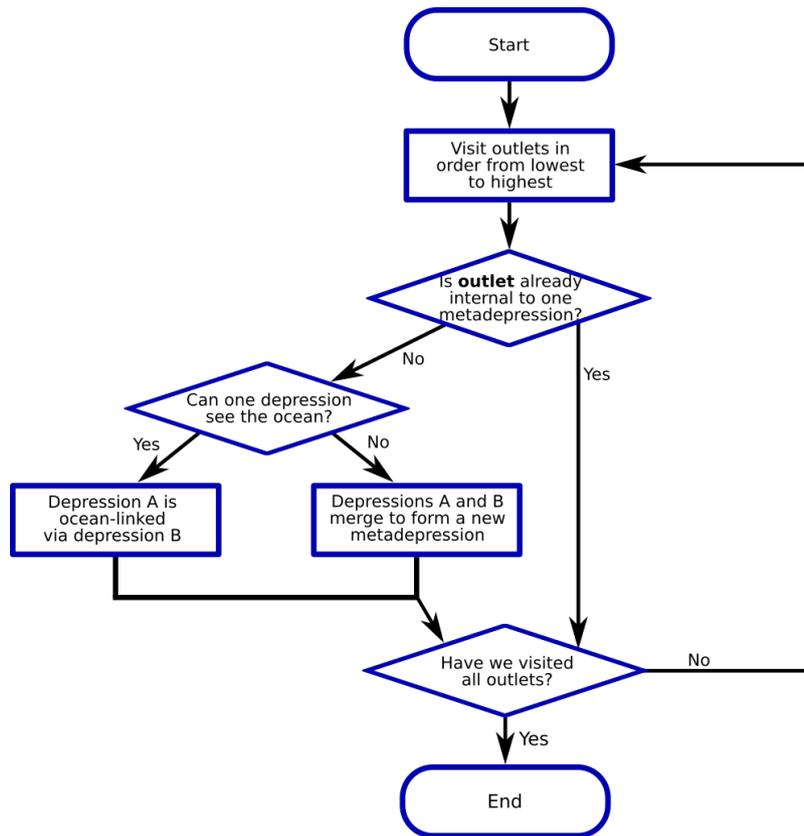
**Figure 6. Construction of the forest of binary trees.** This forest represents the links between individual depressions (Figure 1). See Figure 4 to see how this process fits into the overall depression-hierarchy algorithm.
