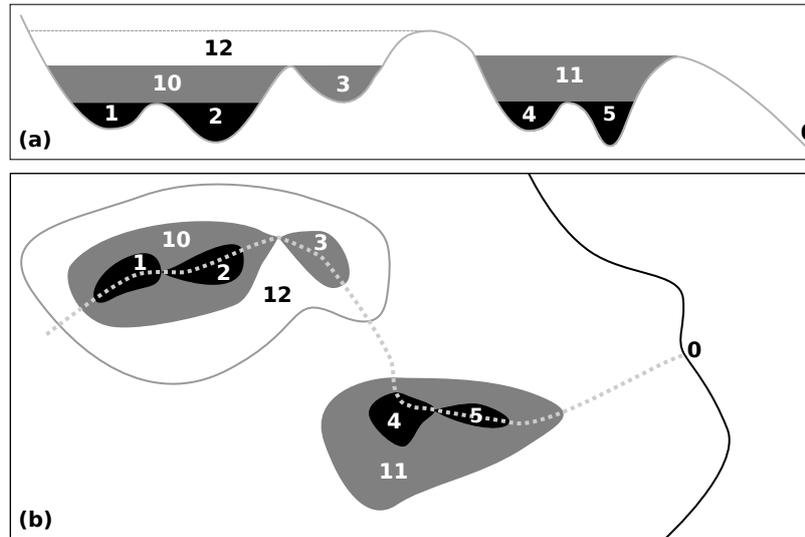
**Figure 3. Cartoon of the left-hand side of the depression hierarchy from Figures 1 and 2.** In this case, we consider depressions to be represented in topography. **(a)** Cross-sectional view. **(b)** Map view. Numbering follows Figures 1 and 2. Flood-fill algorithms used for depression-filling would simply fill these depressions to the highest levels (labelled 11 and 12); the direction of flow and the structure within each depression would not be considered.
