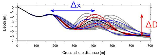
**Figure 2.** Geometry of cross-shore beach profiles used in this study. Different colours are used to highlight that some of the profiles were specifically designed to analyse the effect of variations in the distance or in the relative depth between sandbar crests.
