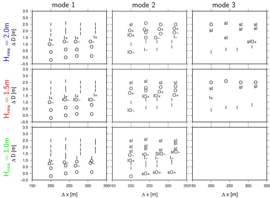
**Figure 7.** Unstable morphological patterns for three unstable modes as a function of  $\Delta D$  and  $\Delta x$ . Each code represents a different pattern (detailed in Figure 6). The top, center and bottom panels represent results obtained for a wave height equal to 1.0, 1.5 and 2.0 m.
