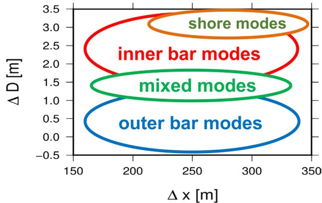
**Figure 9.** Sketch of the most likely fastest growing modes as a function of the geometry of the cross-shore profile.  $\Delta D$  represents the difference between the water depth over the two sandbar crests while  $\Delta x$  is the distance between the two sandbar crests.
