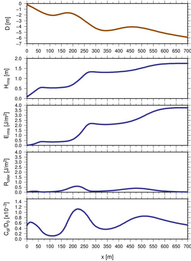
**Figure 3.** Basic state variables for a typical cross-shore beach profile (shoreline is at  $x = 0$ ). From top to bottom: water depth, ~~root-mean square-wave~~ height, ~~wave energydissipation~~, roller energy and depth-averaged sediment concentration.
