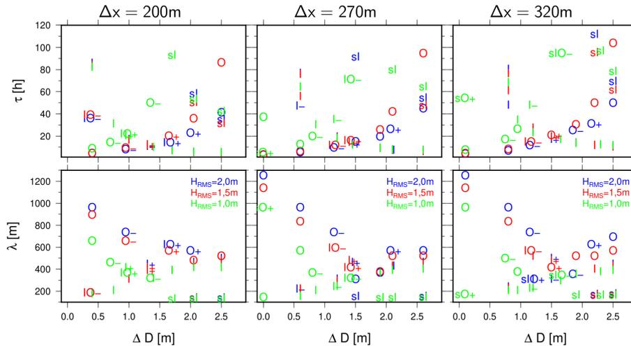
**Figure 8.** Growth time (top) and rip channel spacing (bottom) as a function of  $\Delta D$ . The left, center and right panels represent results obtained for  $\Delta x=200, 270$  and  $320$  m, respectively. Blue, red and green symbols refer to wave height equal to 1.0, 1.5 and 2.0 m.
