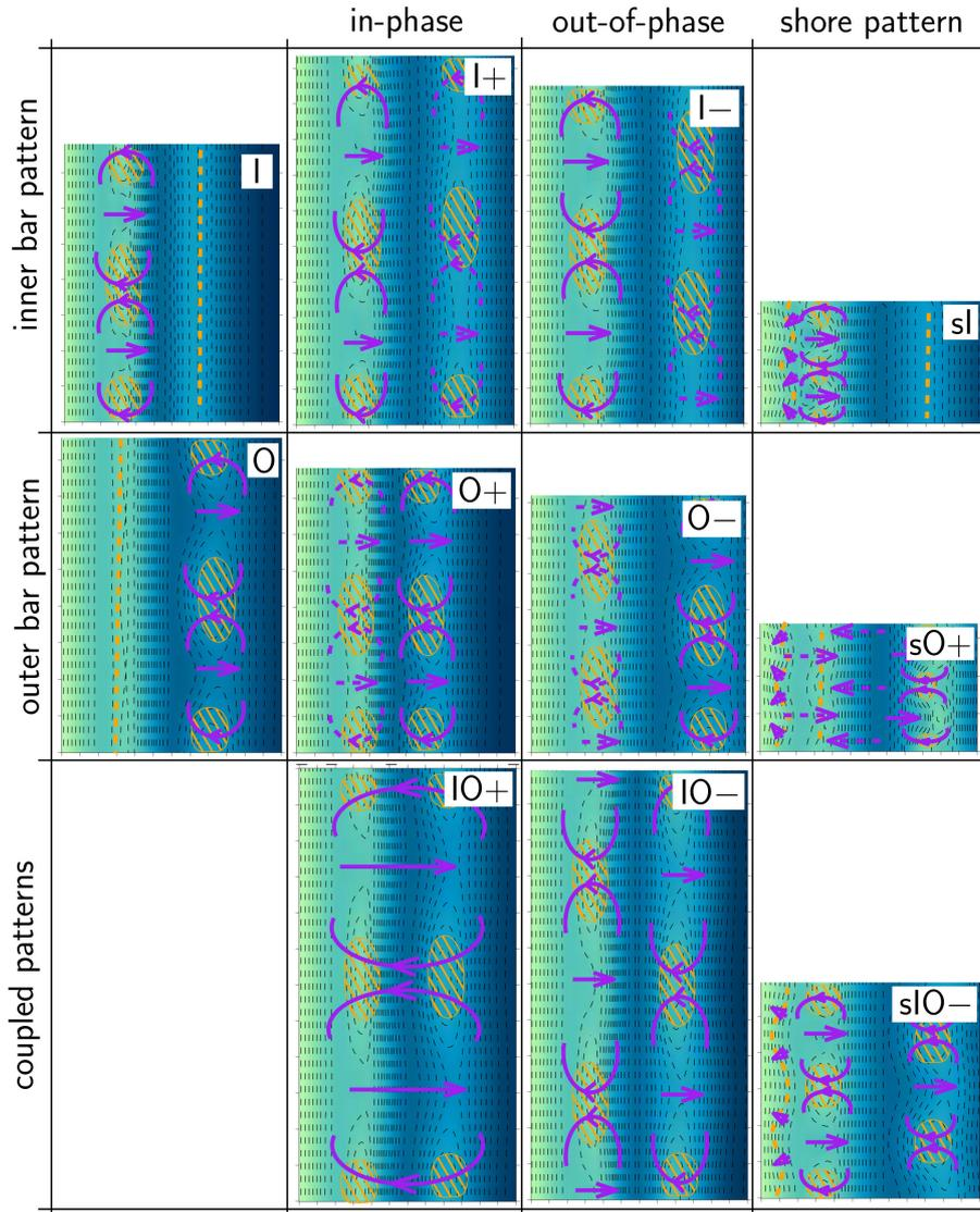
**Figure 6.** ~~Unstable-morphological~~ Morphological patterns obtained in this study. The letters I and O indicate a dominance of the inner and outer sandbar, respectively. Patterns indicated with the code IO ~~represents~~ represents modes where both sandbars are simultaneously unstable. The symbols + and - are used to indicate possible 'in-phase' or 'out-of-phase' coupling. Modes affecting shoreline/inner surfzone morphology have been indicated ~~using~~ by the subscript s.
