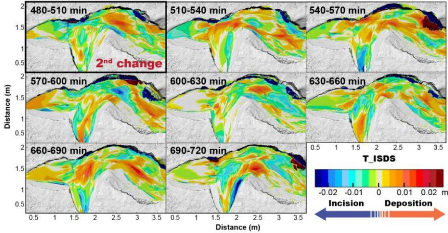
559 Figure 10. Sediment transfer dynamics within the system in the T-ISDS experiment (from DoDs
