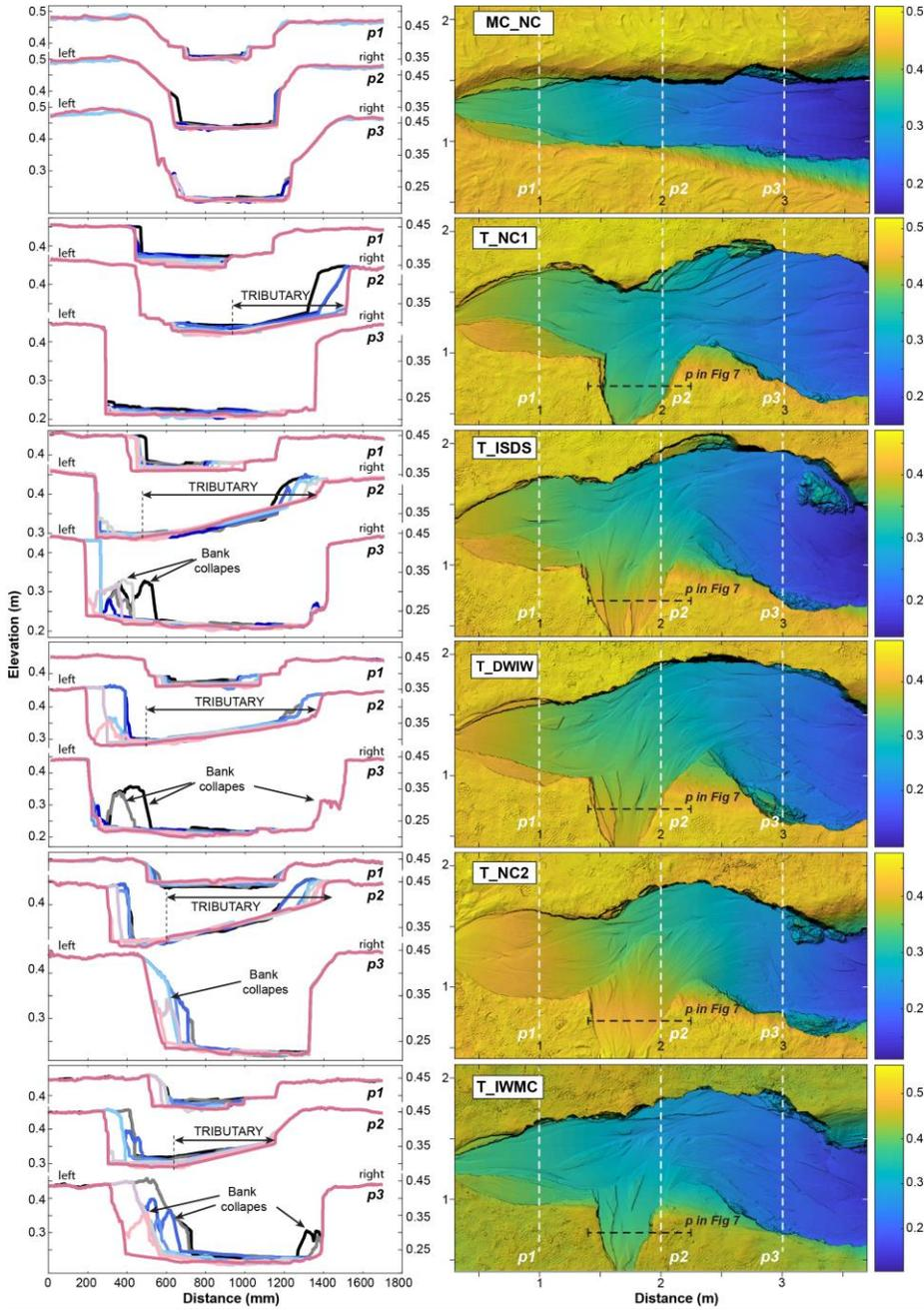
451 Figure 5. Left panels: Cross sections obtained from the DEMs at three different locations along
