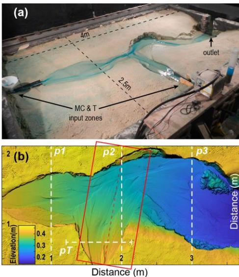
Figure 2. Experimental set-up. (a) Wooden box for the experiments showing the two zones of sediment and water input, and the outlet of the basin. (b) Digital elevation model constructed from laser scans (1 mm horizontal resolution). Red box shows the area of the swath grid used for the calculation of the tributary long profile (Fig. 4) and slope values. Dashed white lines represent the location of the cross sections shown in Figs. 5 and [S1 of the Supplementary Material](#).
