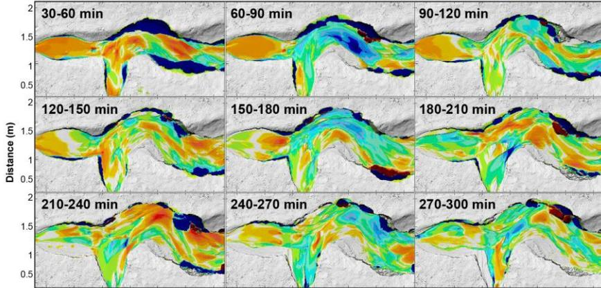
(b) **Increasing sediment** ( $Q_{s\_in\ (TRIBUTARY)} = 4.5\ \text{mL/s}$ )
