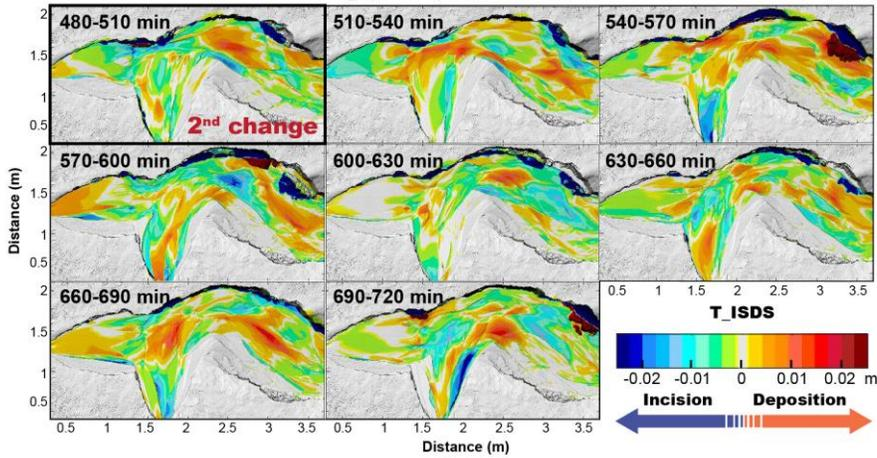
Figure 10. Sediment transfer dynamics within the system in the T\_ISDS experiment (from DoDs analysis). Variations between  $-0.001$  and  $+0.001$  m are considered as “no change” (in gray) to account for the DEMs accuracy (i.e., 1 mm resolution). (a) Pre-perturbation phase (between 30 and 150 minutes is considered to be the spin-up phase); (b) Fan aggradation (300–390 min) and progradation (390–480 min) phase; (c) Fan incision and progradation phase (480 min until end of run).
