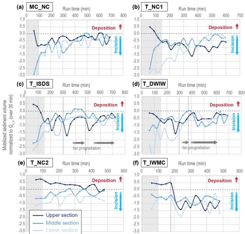
Figure 9f. Volume ( $V$ ) of sediment mobilized in each section (e.g., upper, middle, and lower sections). Vertical lines represent the *times of change* in boundary conditions; horizontal dashed line separates aggradation and erosion.
