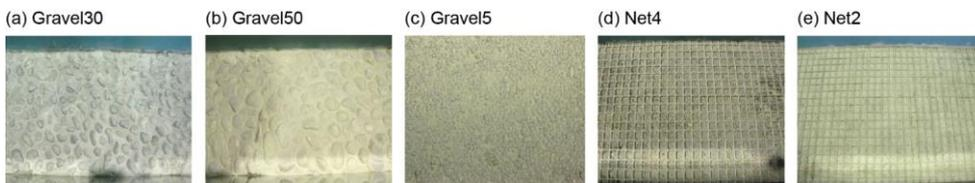
Figure 1: Initial channel bed for each run. (a) Gravel30 is embedded with 30 mm gravel (b) Gravel50 is embedded with 50 mm gravel (c) Gravel5 is embedded with 5mm gravel (d) Net4 is installed with a net of height 4 mm (e) Net2 is installed with a net of height 2 mm.
