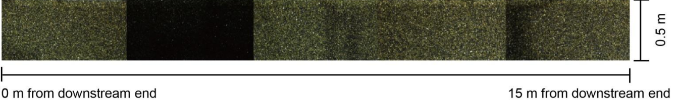
365 Figure 4: Bedrock exposure in Gravel5 series at the end of the experiment. The initial bed had 5mm embedded particles.
