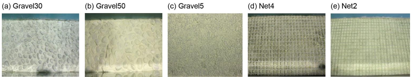
Figure 1: Initial channel bed for each run. (a) Gravel30 is embedded with 30 mm gravel (b) Gravel50 is embedded with 50 mm gravel (c) Gravel5 is embedded with 5mm gravel (d) Net4 is installed with a net of height 4 mm (e) Net2 is installed with a net of height 2 mm.
