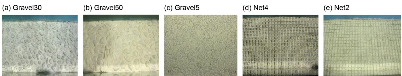
265 Figure 1: Initial channel bed for each run. (a) Gravel30 is embedded with 30 mm gravel (b) Gravel50 is embedded with 50 mm gravel (c) Gravel5 is embedded with 5mm gravel (d) Net4 is installed with a net of height 4 mm (e) Net2 is installed with a net of height 2 mm.
