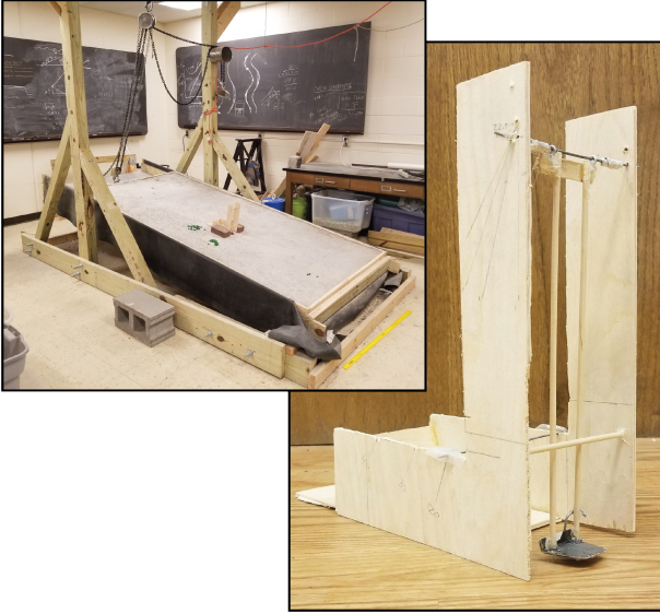
Figure 6. Picture of set-up for travel distance experiments. Left: The experimental hillslope surface is concrete with sand scale roughness. The angle of the slope can be adjusted with a pulley system. Right: Pendulum catapult constructed to deliver particles to the hillslope surface with negligible rotational motion, minimum velocity perpendicular to slope, and known slope-parallel velocity. A gravel-sized particle is placed on the low-friction (glossy cardboard) cradle surface at the base of the 20 cm pendulum arms. A wand is used to gently push the cradle back to a preset angle then quickly removed. The pendulum would be stopped by the wooden bumper rod installed on the frame thus leaving it up to momentum to deliver the particle to the surface. The cradle rests about 2 mm above the surface at its lowest point.
