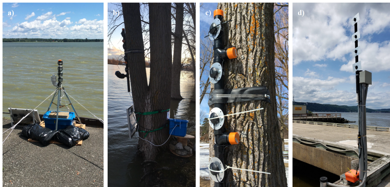
Figure 2. Pictures of antenna arrays a) at Trois-Rivières, b) and c) show different angles at Sainte-Anne-de-Bellevue and d) at Piermont. The antenna array showed in b) and c) was also temporarily installed at Trois-Rivières. The antennas are closer together in a) in comparison to the other two setups.
