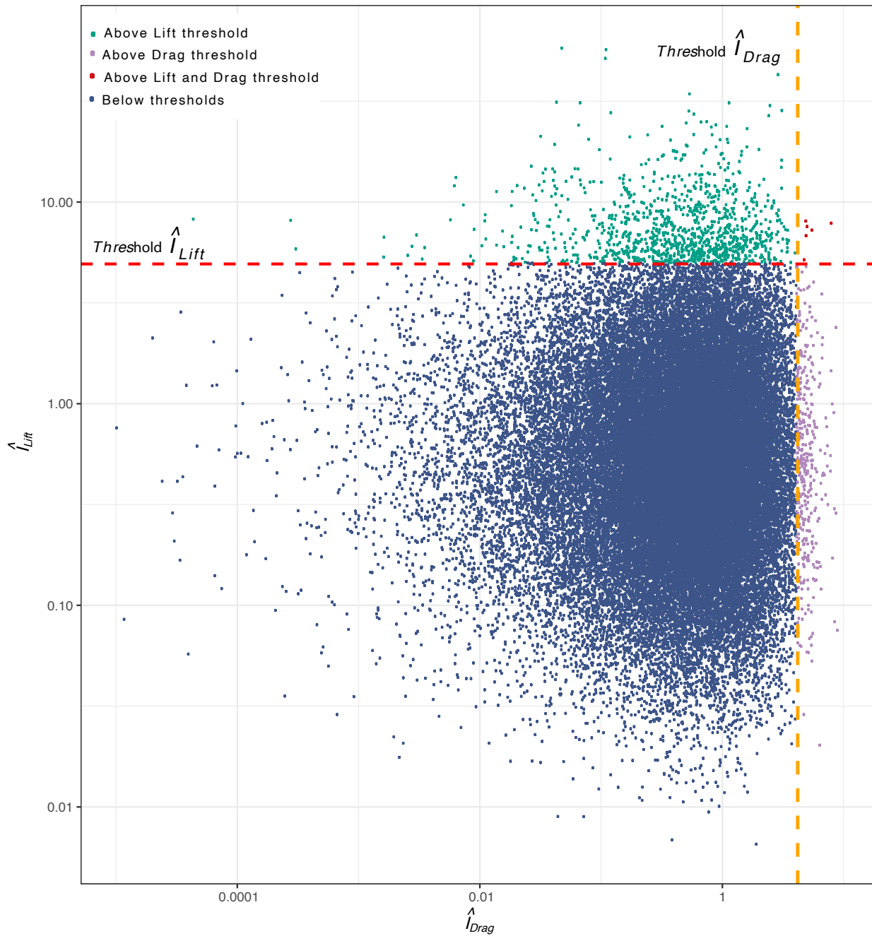
Figure 7. Bootstrap normalised impulse sampling (lift and drag). \hat{I}_{Drag} and \hat{I}_{Lift} are fitted with a gamma and a log-normal distribution, respectively (Appendix F2). The normalised drag and lift thresholds (red dashed lines), are calculated using the probabilistic drag and lift inertial impulse thresholds presented in Figure 5 which were divided by the recorded mean inertial drag and lift impulse from the laboratory experiments.
