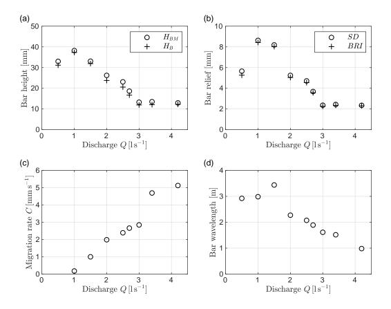
Figure 3. Mean properties of bars depending on discharge: (a) bar height  $H_{BM}$  and  $H_B$ ; (b) bed relief, as measured by the standard deviation of the bed elevation distribution (SD) and the bed relief index (BRI); (c) bar migration rate C; (d) bar wavelength L.
