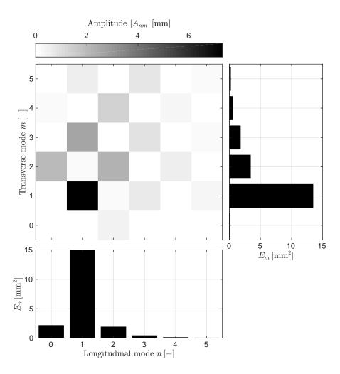
Figure 8. Amplitude of the first  $6 \times 6$  longitudinal and transverse modes for the ensemble bar at  $Q = 2.51 \,\mathrm{s}^{-1}$ . Histograms on the bottom and on the left also reports the total energy  $E_n$  and  $E_m$ , representing the variance of the bed elevation associated with all the components having longitudinal mode n and transverse mode m, respectively.
