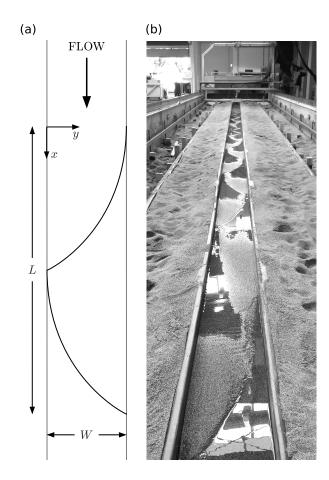
Figure 1. (a) reference system (x,y) for and individual bar of wavelength L in a straight channel of width W, with the curved line indicating the typical position of bar fronts; (b) picture of the flume at the end of the experiment with  $Q=2.51\,\mathrm{s}^{-1}$ , showing the presence of alternate bars. Flow is from top to bottom.
