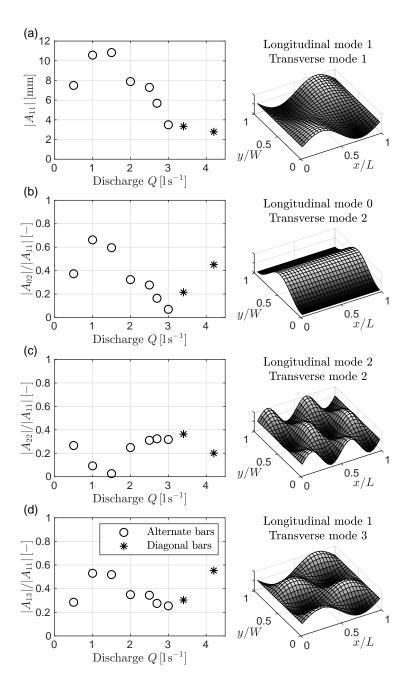
Figure 9. Amplitude of the main Fourier components depending on discharge. (a): amplitude of the fundamental harmonic  $(A_{11})$ ; (b), (c) and (d): ratio between the amplitudes  $A_{02}$ ,  $A_{22}$ ,  $A_{13}$  and the fundamental. The 3-D plots on the right illustrate the bed deformation associated with each Fourier component.
