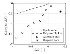
**Figure 7.** Skewness of the bed elevation distribution as a function of the scaled discharge. Markers indicate the skewness of the experimental ensemble bars; lines illustrate results from the weakly nonlinear theory, with the dash-dot line referring to the solution obtained by limiting the bar growth to the fully-wet condition.
