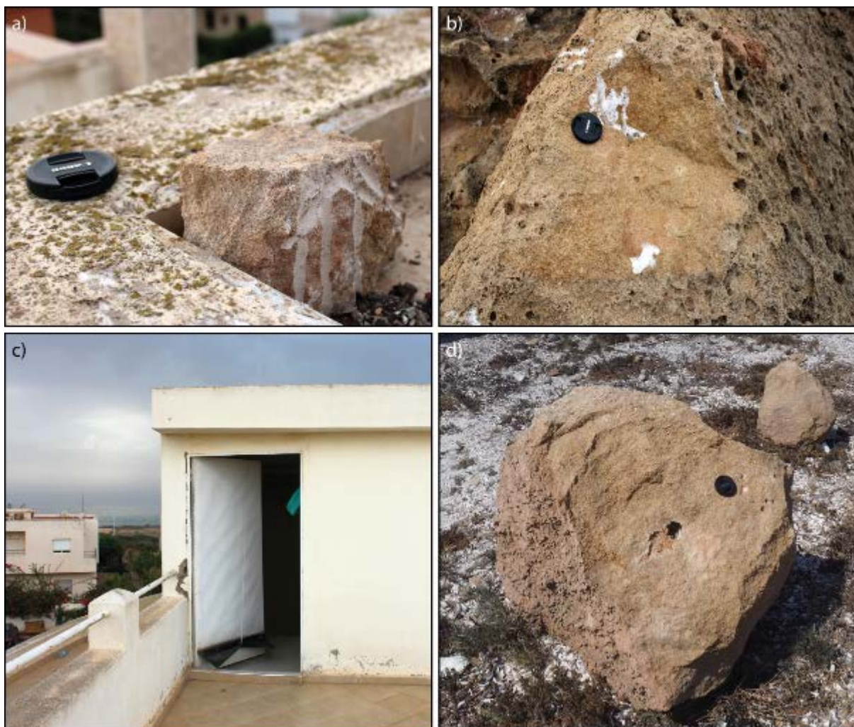
Fig. A16: Calibration samples. a) Roof top sample VAL 4-1 CAL I. b) Surface on boulder VAL 4 exposed during first field survey in July 2016 by removing at least 10 cm of rock. c) Roof of the house used for artificially exposing rock samples; samples VAL 4-1 CAL I and HAR 1-1 CAL were placed on top of the highest roof shown in the photo. d) Surface of boulder TEM 3 exposed during the first field survey in July 2016; at least 10 cm of rock were removed.
