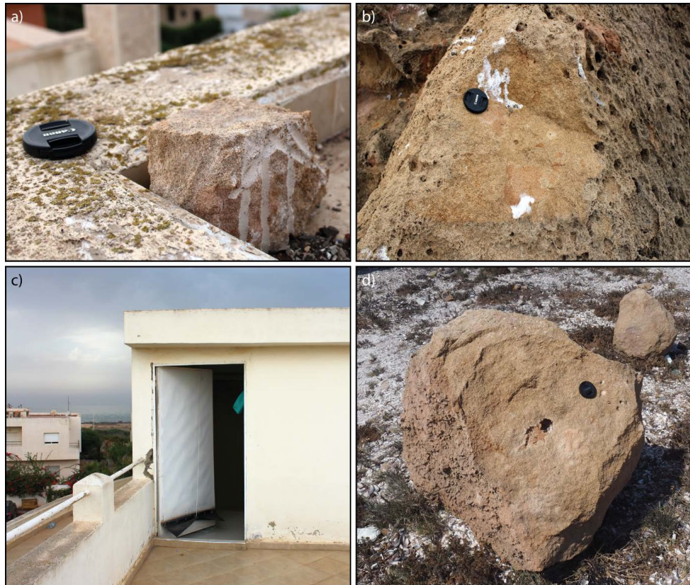
Fig. A17: Calibration samples. a) Roof top sample VAL 4-1 CAL I. b) Surface on boulder VAL 4 exposed during first field survey in July 2016 by removing at least 10 cm of rock. c) Roof of the house used for artificially exposing rock samples; samples VAL 4-1 CAL I and HAR 1-1 CAL were placed on top of the highest roof shown in the photo. d) Surface of boulder TEM 3 exposed during the first field survey in July 2016; at least 10 cm of rock were removed.
