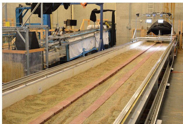
Figure 2. Adjustable-Boundary Experimental System (A-BES) at the University of British Columbia, showing the camera rig and the 30 cm wide channel configuration.
