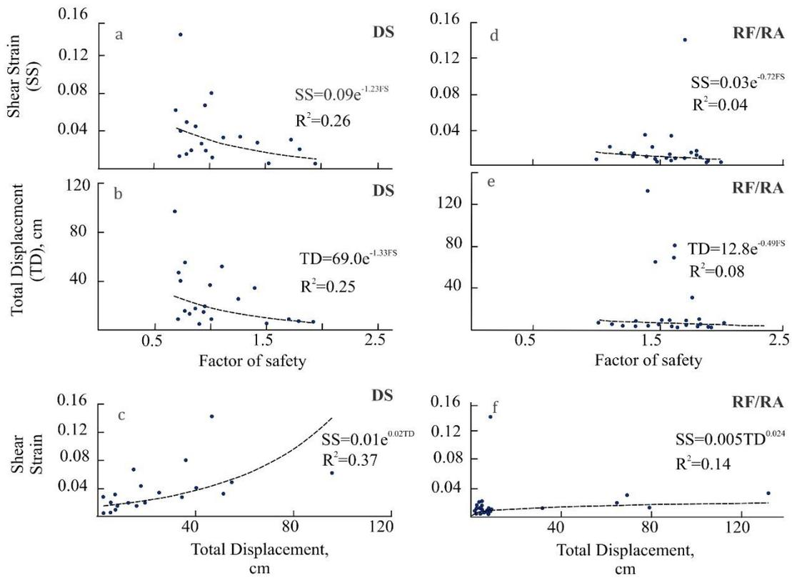
**Fig. 5** Relationship of Factor of Safety (FS), Total Displacement (TD) and Shear Strain (SS).
