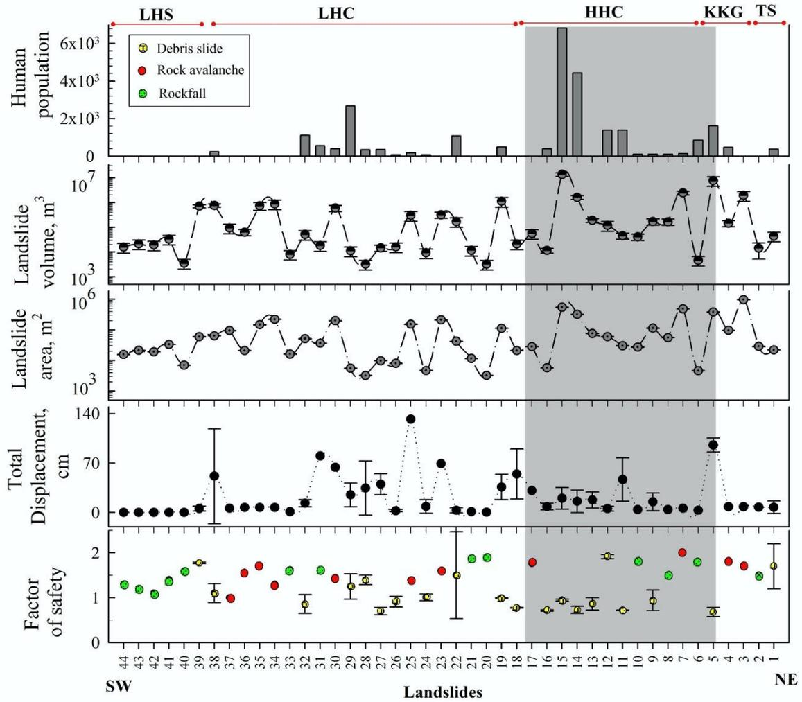
**Fig. 4** The FEM analysis of all forty-four landslides. Grey bar in the background highlights the Higher Himalaya Crystalline (HHC) region that comprises relatively more unstable landslides, ~~relatively more~~ landslide volume and human population. ~~Source of human population: Census 2011 (Govt. of India, New Delhi).~~ TS, KKG, HHC, LHC and LHS are Tethyan Sequence, Kinnaur Kailash Granite, Higher Himalaya Crystalline, Lesser Himalaya Crystalline and Lesser Himalaya Sequence, respectively
