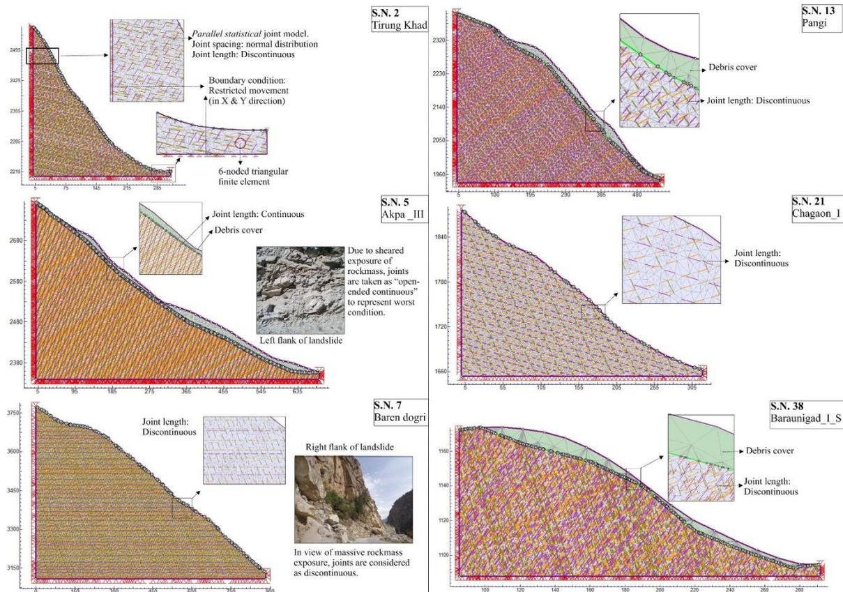
**Fig. 3** The FEM configuration of some of the slope models. S.N. refers to the serial no. of landslides in Table 1. The joint distribution in all the slopes was parallel-statistical with the normal distribution of joint spacing.
