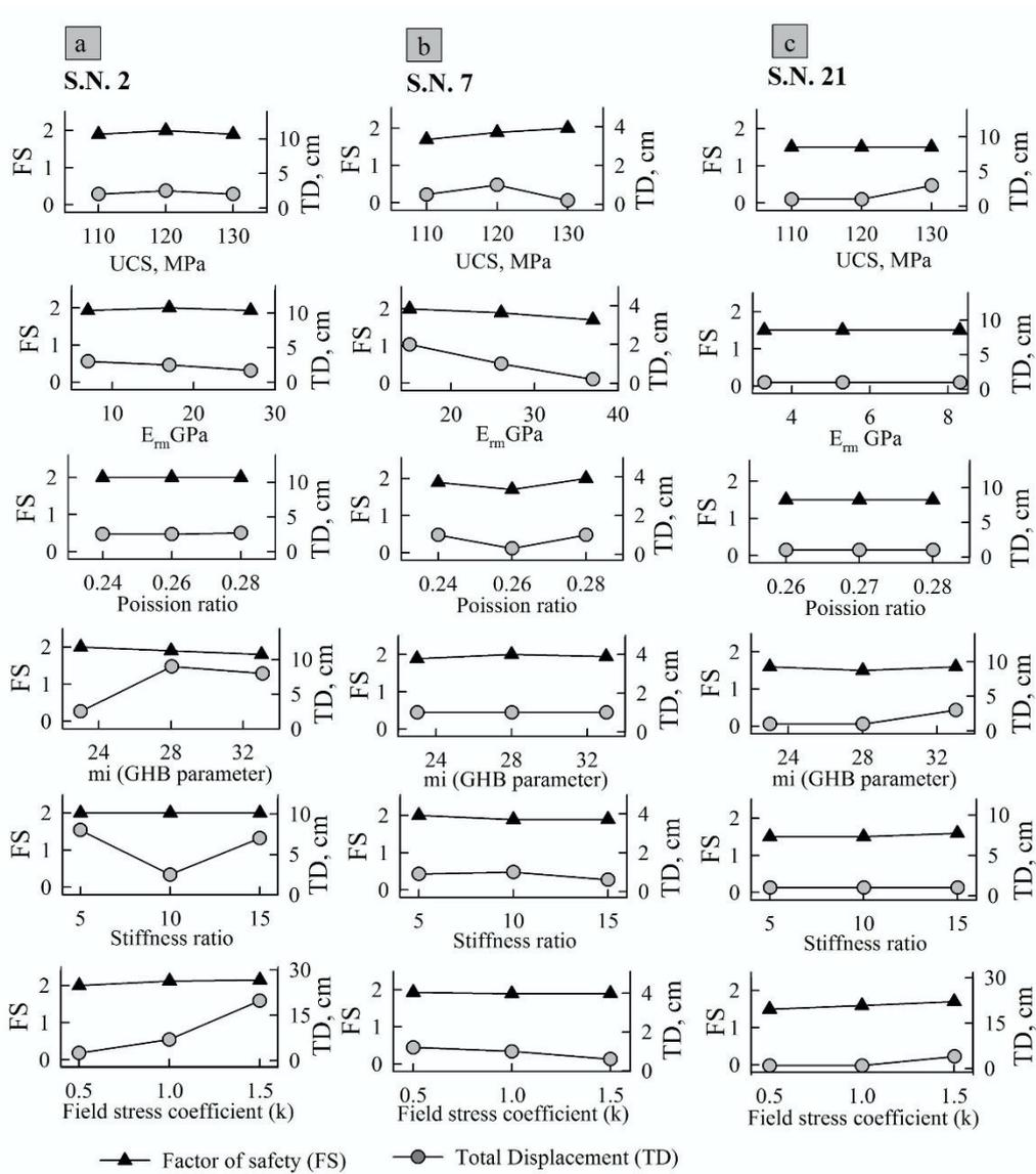
**Fig. 7** Parametric analysis of rockfall/rock avalanche. (a) Tirung khad (S.N. 2); (b) Baren Dogri (S.No. 7); (c) Chagaon\_II (S.N. 21).
