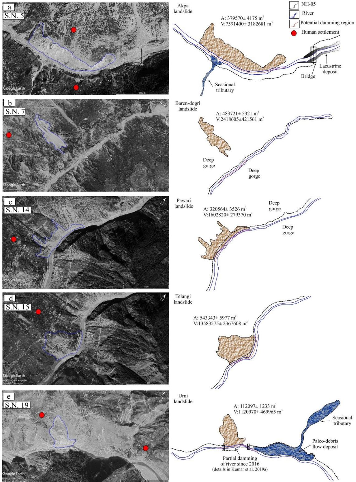
**Fig. 9** Potential landslide damming locations. (a) Akpa\_III landslide; (b) Baren dogri landslide; (c) Pawari landslide; (d) Telangi landslide; (e) Urni landslide.
