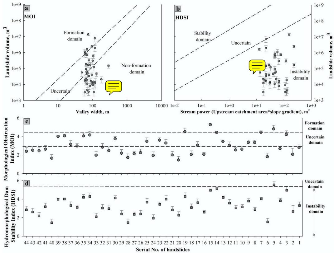
**Fig. 8** Landslide damming indices (a) Morphological Obstruction Index (MOI); (b) Hydro-morphological dam stability index (HDSI); (c) Landslides vs. MOI; (d) Landslides vs. HDSI.
