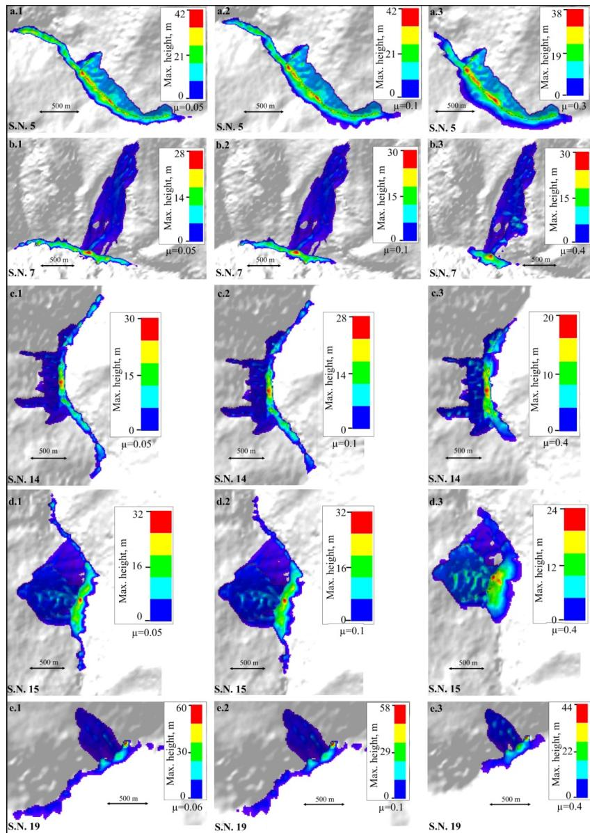
**Fig. 13** Results of run-out analysis.  $\mu$  refers to coefficient of friction. S. N. refers to serial no. of landslides in Table 1
