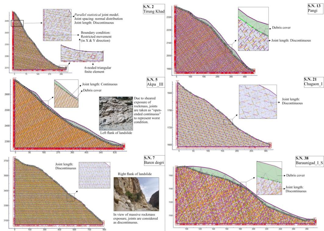
**Fig. 3** TheFEM configuration ofsome of the slope models. S.N. refers to serial no. of landslides in Table 1. The joint distribution model in all the slopes was parallel statistical with normal distribution of joint spacing.
