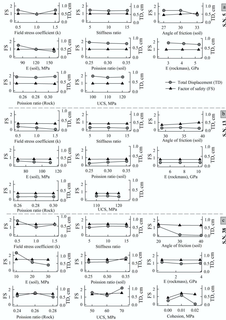
**Fig. 6** Parametric analysis of debris slides. (a) Akpa\_III (S.N. 5); (b) Pangi\_III (S.N. 13); (c) Barauni Gad\_I\_S(S.N. 38). S. N. refers to serial no. of landslides in Table 1.
