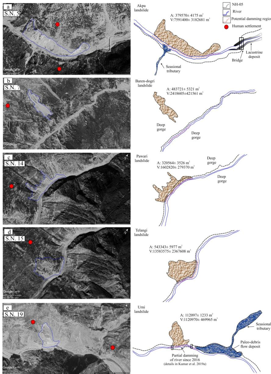
**Fig. 9** Potential landslide damming locations. (a) Akpa III landslide; (b) Baren dogri landslide; (c) Pawari landslide; (d) Telangi landslide; (e) Urni landslide. S. N. refers to serial no. of landslides in Table 1.
