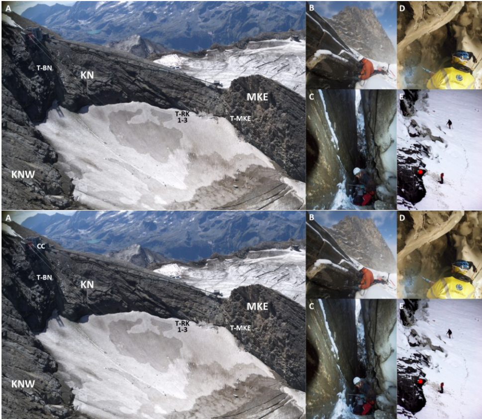
Figure 5: Deep and shallow borehole temperature monitoring at Kitzsteinhorn. 5A : Overview image-Air photo (photo: R. Delleske, 24.08.2017); 5B : Measurement site at the Randkluft aperture (T-RK1) (photo: I. Hartmeyer: 04.09.2015); 5C : Measurement site inside Randkluft, 7 m below the 2015 glacier surface (T-RK2) (photo: R. Delleske, 04.09.2015); 5D : Measurement site inside Randkluft, 14 m below glacier surface (T-RK3) (photo: M. Dörfler, 21.09.2018); 5E : Close-up View of the investigated Randkluft from the cable car top station (CC); red dot indicates position of T-RK1 (photo: F. Miesen, 04.09.2015 6 ).
