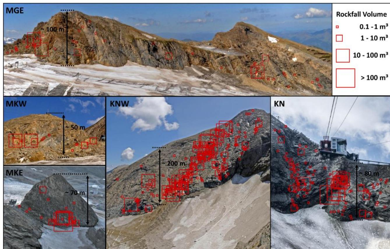
235 **Figure 4: Rockfall source areas and volumes for all five monitored rockwalls. A clear linear distribution along major joint intersections is evident at all rockwalls and is particularly apparent at KNW (Kitzsteinhorn northwest-face) and KN (Kitzsteinhorn north-face) (Photos: Robert Delleske).**
