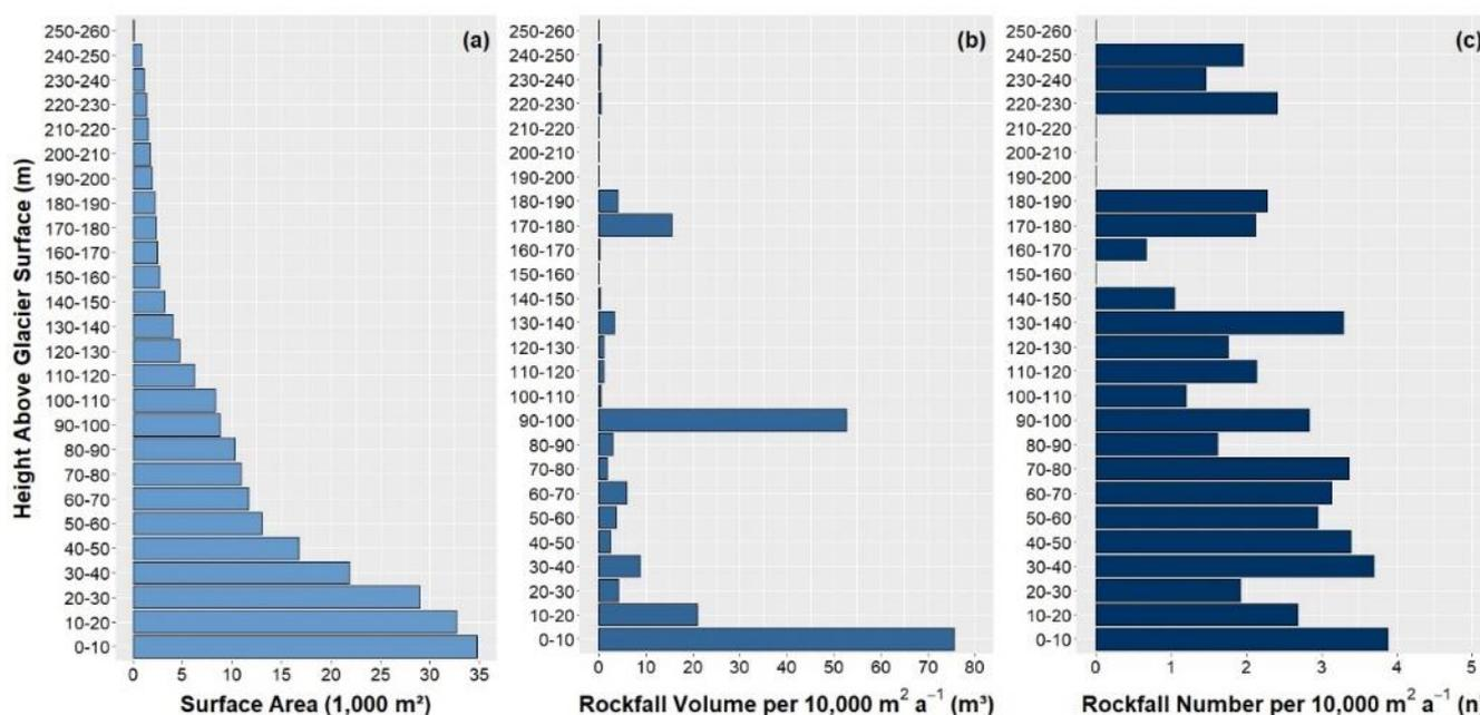
300 **Figure 7: (a) Rockwall surface area, (b) normalized rockfall volume and (c) the normalized number of rockfalls, classified by elevation above glacier surface. Areas exposed by recent glacier retreat are heavily susceptible to rockfall, during the observation period (2011-2017) 60 % of the total rockfall volume detached within 10 m of the current glacier surface.**
