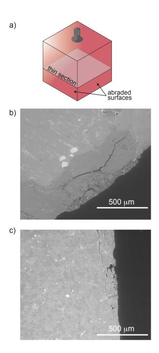
**Figure 4.** Thin section preparation and SEM images. (a) Schematic drawing showing location in grain where thin sections were made. (b) SEM image of quartz diorite. (c) SEM image of volcaniclastic rock.
