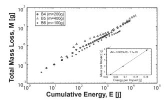
**Figure 6.** Attrition rate for bricks with different collision energies. Plot of total cumulative mass abraded versus cumulative impact energy for three sets of brick with different masses. Inset displays plot of average mass abraded per impact versus average energy per impact. Each data point corresponds to a separate set of bricks.
