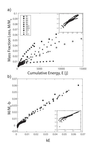
**Figure 5.** Attrition mass loss curves. (a) Plot of total cumulative mass loss versus cumulative impact energy for each set of rocks. (b) Plot of total cumulative mass loss minus y-intercept, b (eq. 7), from linear fits to raw data in (a) versus cumulative impact energy multiplied by value of fit slope. Insets for both (a) and (b) displays plots with log-log axes.
