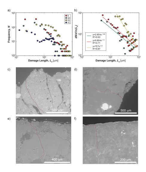
**Figure 8.** SEM results. (a) Plot of the distribution of length of damage within abraded rocks from SEM images of thin sections. (b) Damage lengths plotted in the form of the eq. (6) with corresponding power-law fits. (c)-(f) SEM images of the largest crack length for each rock type outlined in red. (c) Brick (d) Quartz diorite (e) Sandstone (f) Volcaniclastic rock
