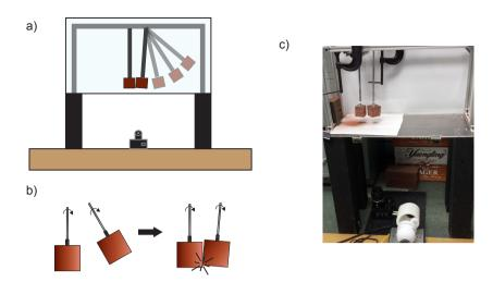
**Figure 1.** Schematic of experimental set-up. (a) Front view drawing depicting binary collisions double-pendulum apparatus. (b) Close-up drawing illustrating how grains impact during collision. The impacting grain is raised then released, colliding with the stationary target grain. Both grains are able to rotate freely. (c) Picture of set-up with brick clasts.
