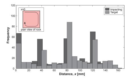
Figure 2. Randomness test for collision rotation. Plot showing the histogram of impact locations for impacting and target grains. Peaks correspond to corners of the cuboid grains. Inset shows plane view of square rock with labeled location of x = 0 at one of the corners and subsequent corners at x = 40 mm, x = 80 mm, and x = 120 mm.
