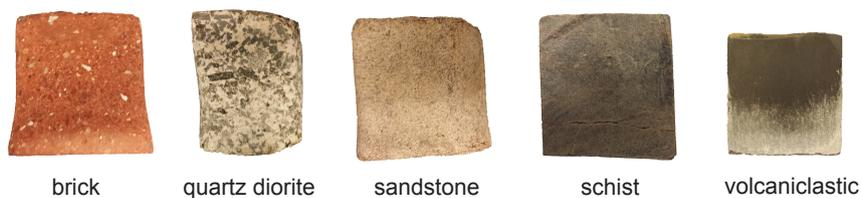
**Figure 3.** Images of samples. Images of all rocks used in the experiments. Images taken at the end of each experiment so there is noticeable rounding of the edges.
