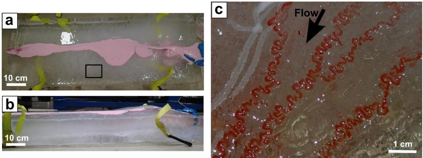
**Figure 3** (a) Top and (b) side view of ice block over which (c) first set of mm-scale self-formed meltwater meanders were observed. Area shown in (c) corresponds to region indicated in (a). Images in (a) and (b) were taken before adding dye.
