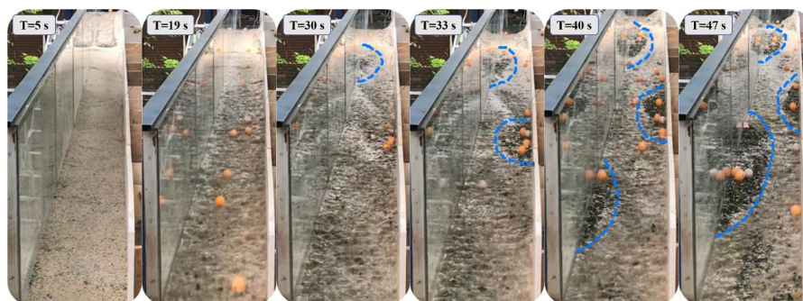
241 242 Figure. 3 The riverbed morphology at six different moments during the sandbars' formations and 243 growths for the T7 experiment. The sandbars in the figure are marked with blue dotted lines.
