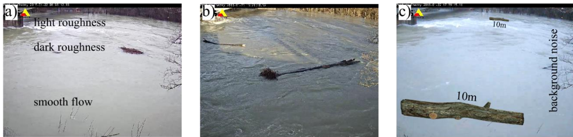
Fig 8 Different light conditions during a) morning, b) noon and c) late afternoon, results in different frame roughness's and different detection performances. c) Wood position can highly affect the quality of detection. Pieces that are passing in front of the camera are detected much better than the pieces far from the camera.
