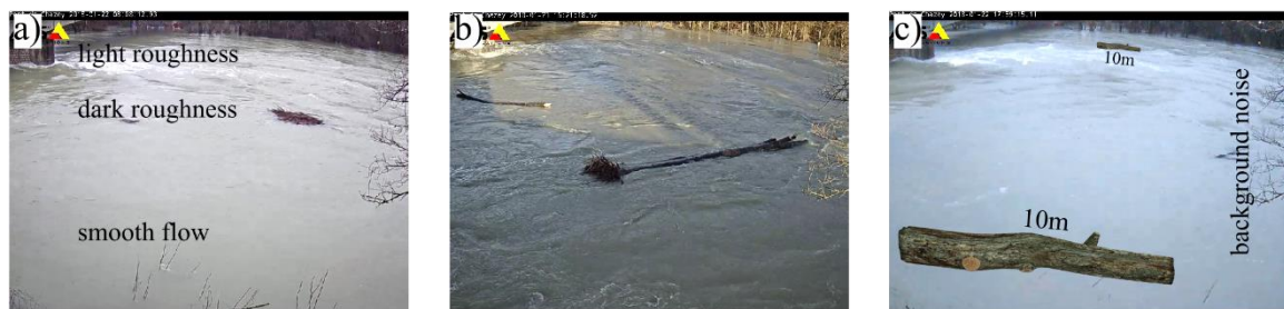
Fig 8 Different light conditions during a) morning, b) noon and c) late afternoon, results in different frame roughness's and different detection performances. c) Wood position can highly affect the quality of detection. Pieces that are passing in front of the camera are detected much better than the pieces far from the camera.
