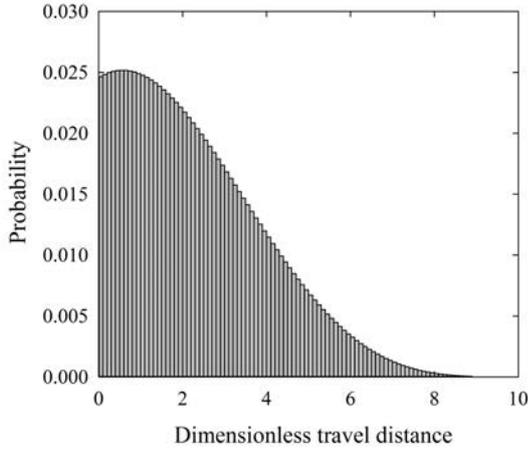
**Figure 7.** Probability mass function  $f_k(k; \hat{x})$  of discrete travel distances  $k$  associated with initial net heating over small  $k$  followed by net cooling with increasing  $k$ , leading to a finite mode. In this example the Kirkby number starts at  $Ki = 0.90$  at  $k d \hat{r} = \hat{x} = 0$  and decreases to  $Ki = 0.57$  at  $k d \hat{r} = \hat{x} = 10$ .
