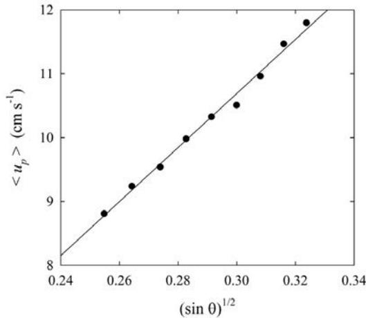
**Figure J1.** Plot of ensemble averaged particle velocity  $\langle u \rangle$  versus  $\sqrt{\sin \theta}$  involving a steel sphere ( $R = 2.5$  mm) moving over glass beads ( $r_m = 0.53$  mm) giving  $R/r_m = 4.7$ ; data from Samson et al. (1998).
