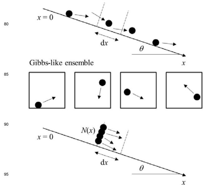
**Figure B1.** Schematic diagram of surface inclined at angle  $\theta$  and control volume with edge length  $dx$  through which particles move, with Gibbs-like ensemble of single-particle systems leading to definition of the cohort of  $N(x)$  particles starting at the left face of the control volume.
