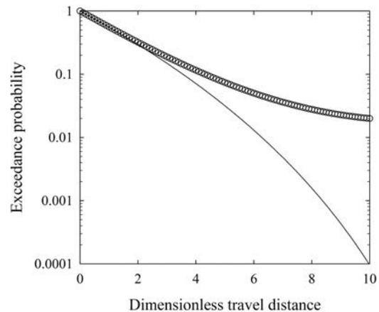
**Figure 6.** Plot of exceedance probability  $R_{\hat{x}}(\hat{x})$  versus dimensionless travel distance  $\hat{x}$  showing conditions with fixed net cooling (solid line) and conditions that start with the same cooling rate but then involve a decreasing rate with increasing distance  $\hat{x}$  (circles). In this example the Kirkby number starts at  $Ki = 0.70$  at  $\hat{x} = 0$  and increases to  $Ki = 0.96$  at  $\hat{x} = 10$ .
