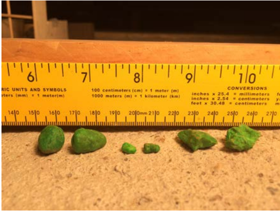
Figure 7. Image of rounded (left), small (center) and angular (right) test particles on the concrete surface with granular roughness texture.
