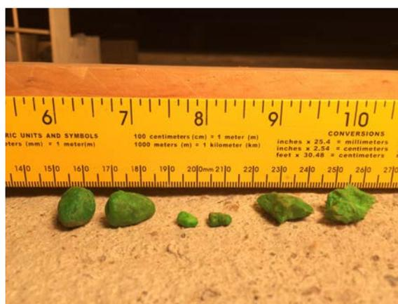
**Figure 7.** Image of rounded (left), small (center) and angular (right) test particles on the concrete surface with granular roughness texture.
