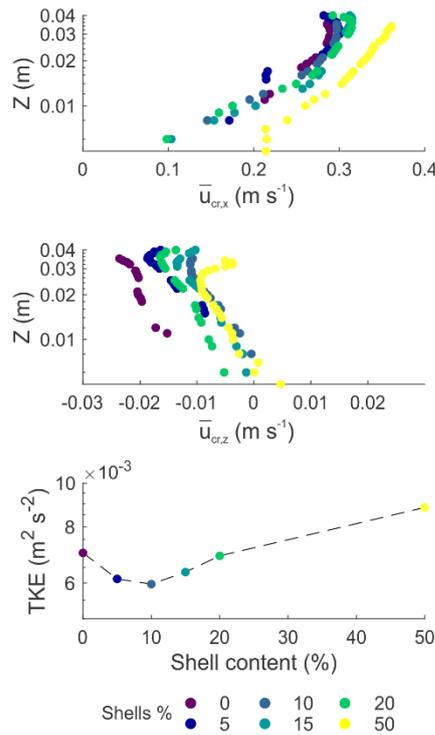
**Figure 5:** Time-averaged near-bed velocity profiles showing the (a) x and (b) z direction of the constant flow experimental runs, as well as the (c) the peak TKE profiles values plotted against shell content. *Note:* The profiles are time-averaged, as indicated by the overbars, over the entire duration of each experimental run.
