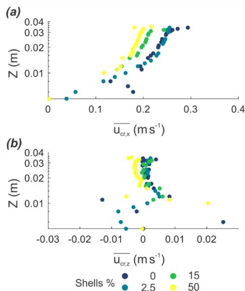
**Figure 6:** (a) Near-bed ~~horizontal streamwise flow and~~; (b) vertical flow ~~and~~ (c) TKE profiles at the onset of sediment transport for flat beds (ACC flow experiment). *Note:* The overbars denote that the x-axes ~~The profiles are time-averaged,~~ over a 10-minute period, which encompasses the 5 minutes prior to and following the incipient motion, for the four selected experimental runs.
