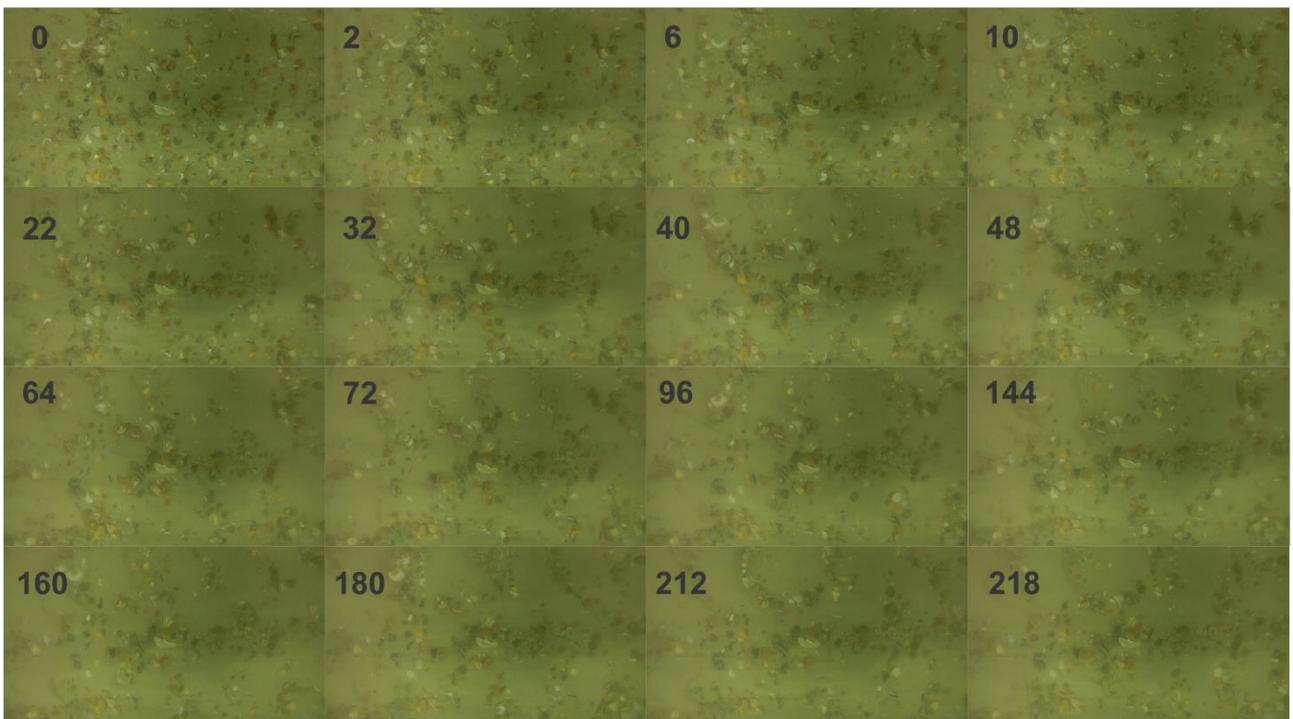
**Figure S2:** [Snapshots extracted from the GoPro footage of the constant flow experiment to show that the majority of the shells remain in place throughout the duration of experimental run at both the low and high shell treatments.](#)
