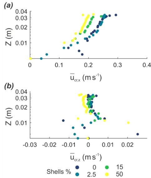
**Figure 6:** (a) Near-bed horizontal streamwise flow and (b) vertical flow profiles at the onset of sediment transport for flat beds (ACC flow experiment). Note: The overbars denote that the x-axes are time-averaged over a 10-minute period, which encompasses the 5 minutes prior to and following the incipient motion, for the four selected experimental runs.
