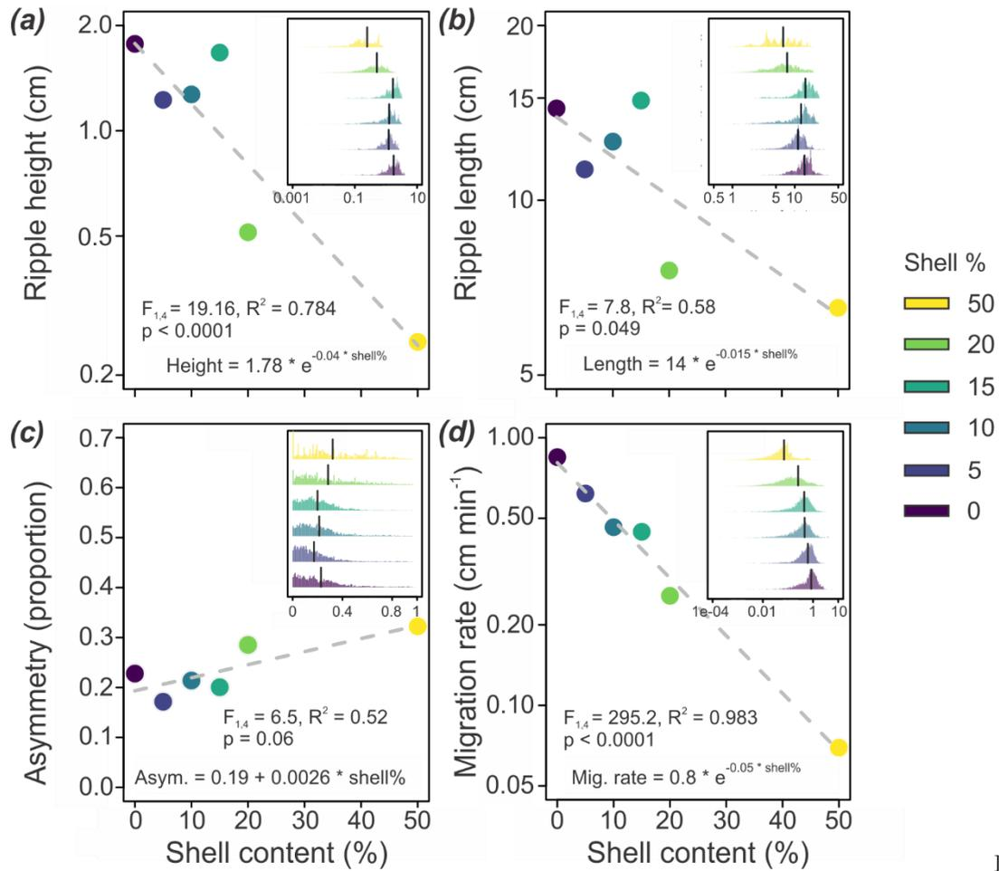
Figure 4: (a) Ripple height, (b) Ripple length, (c) Asymmetry and (d) Migration rate, plotted against the shell content from the constant flow experimental runs ( $n = 6$ ). The y-axis of the ripple height, length and migration are plotted under a log scale. *Inset panels:* The corresponding histograms for each ripple parameter, with the x-axis values representing the y-axis values of the respective regression plots. Vertical lines represent mean values.
