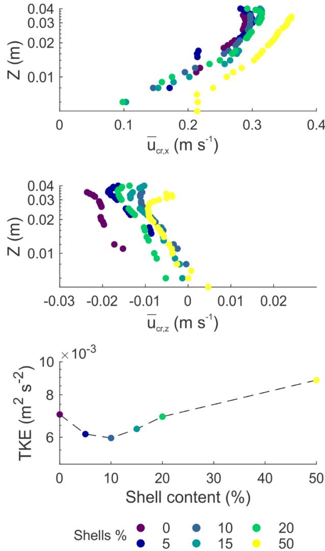
285 **Figure 5: Time-averaged near-bed velocity profiles showing the (a) x and (b) z direction of the constant flow experimental runs, as well as the (c) peak TKE values plotted against shell content. Note: The profiles are time-averaged, as indicated by the overbars, over the entire duration of each experimental run.**
