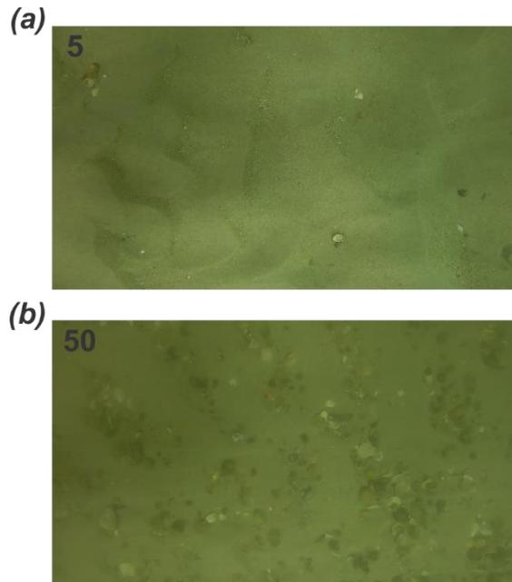
260 **Figure 3: Stills taken from the GoPro videos (constant flow experiment) to show the contrast between a (a) low-density and (b) high-density treatment. Shells increasingly appear as immobile clusters at higher concentrations, as they are periodically exposed due to sand movement. The numbers represent the shell %.**
