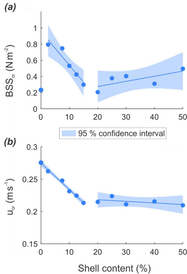
**Figure 7: (a): The critical BSS for incipient motion and the (b) corresponding depth-averaged velocity for the ACC flow experiment. The shaded regions represent the 95<sup>th</sup> percentile confidence intervals.**
