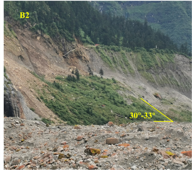
Fig. S6: The slope angles of some PSF in field investigation, photographs by Yan Zhong.
