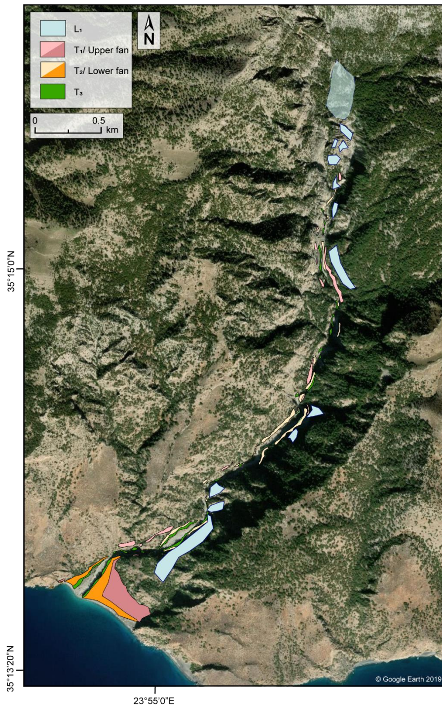
Figure S4: Full-valley mapping of sedimentary deposits and landslide deposits. All deposits are distributed along the valley's entire length, suggesting a shared place of origin in the headwaters. For more mapping details of the terrace and fan deposits, see Booth (2010).
