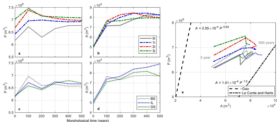
335 **Figure 10: The evolution of tidal prism, inlet cross-sectional area and “P-A relation” for the different mouth island scenarios over 500 years. (a) and (b) for the scenarios of different number of mouth islands, (c) and (d) for the scenarios of different location of mouth islands.**
