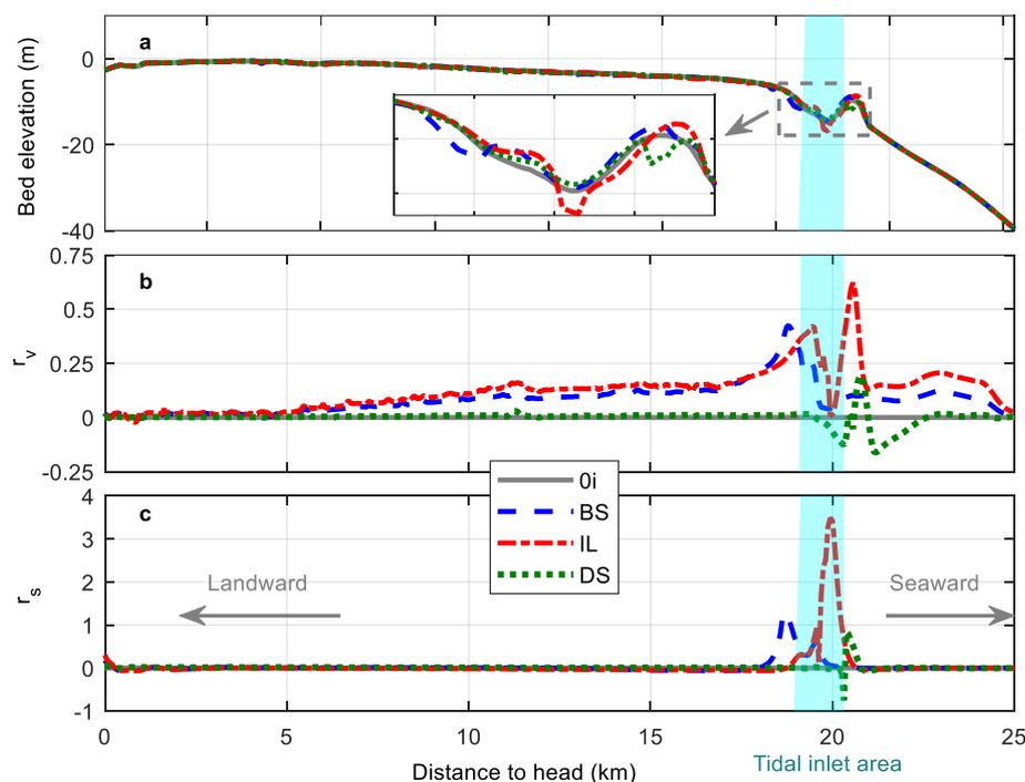
435 **Figure 14: Longitudinal variations of cross-sectionally averaged bed elevation after 500 years (a), flow velocity at the beginning (b) and sediment transport at the beginning (c) compared to the case of zero island.**
