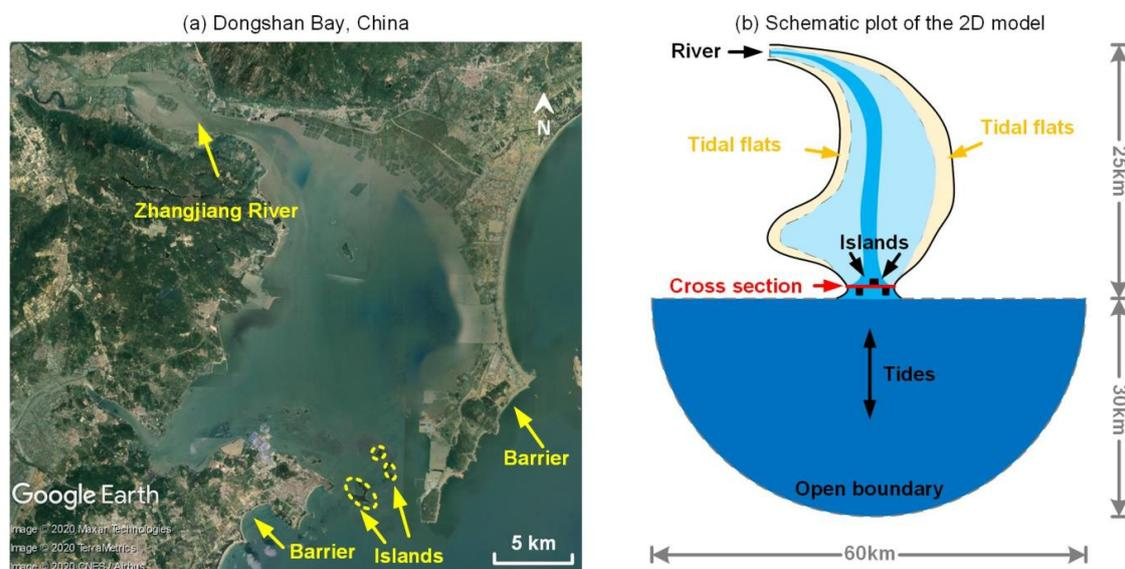
**Figure 2:** (a) The reference barrier basin with three mouth islands near the inlet, Dongshan Bay (23° 49' 48" N, 117° 31' 18" E; Image © 2020 Google Earth, Maxar Technologies); (b) The schematized model domain used in this study.
