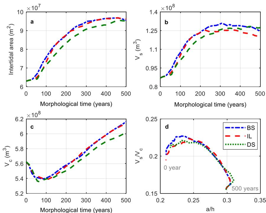
390 **Figure 12: Temporal variation of intertidal flat area (a), intertidal storage volume (b), channel volume (c) and ratio of  $V_s/V_c$  in the inner basin of different island locations.**
