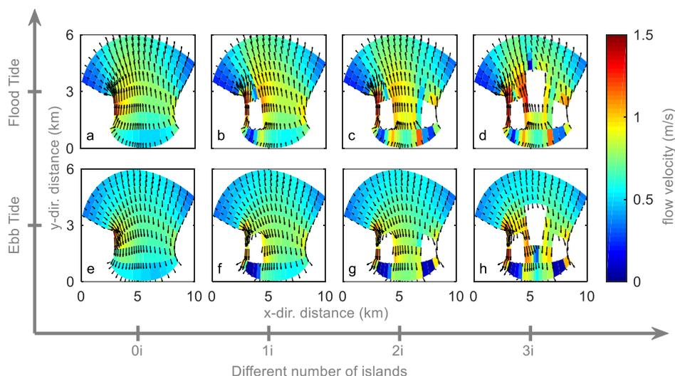
200 **Figure 5: Flow field near the inlet: (a-d) represent at the time of flood tide of basin without island (“0i”), basin with one island (“1i”), basin with two islands (“2i”) and basin with three islands (“3i”) and (e-h) represent at the time of ebb tide respectively. Arrows for flow direction and colour for depth-averaged flow velocity (m/s).**
