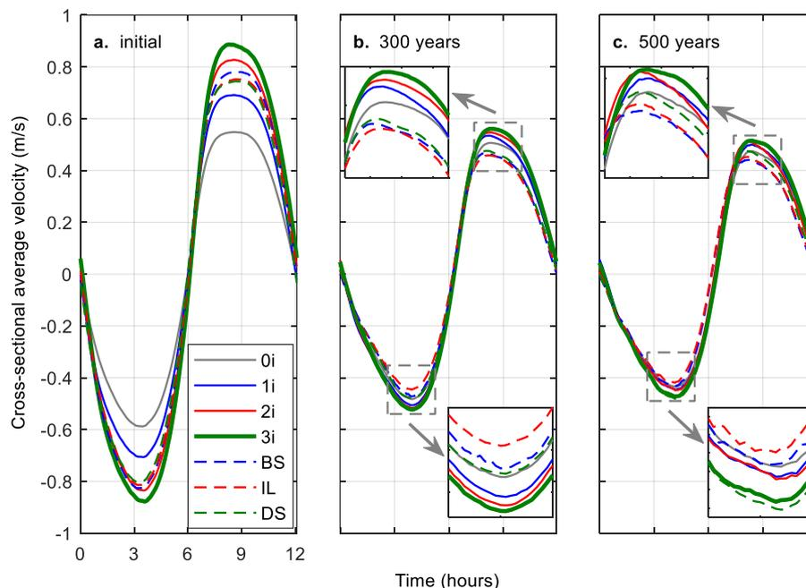
365 **Figure 11: The cross-sectional average velocity over a tidal cycle of different scenarios after: (a) 0 years, (b) 300 years, and (c) 500 years. The flood tidal velocity is positive.**
