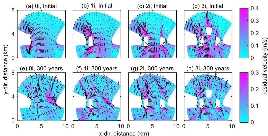
250 **Figure 7: Spatial distribution of the residual current (arrow vectors indicate the direction) near the tidal inlet of four different scenarios: (a-d) represent without island (0i), one island (1i), two islands (2i) and three islands (3i) at the beginning respectively. (e-h) after 300 years. The white area in the plot represents the mouth islands and the background color represent the magnitude of residual velocity.**
