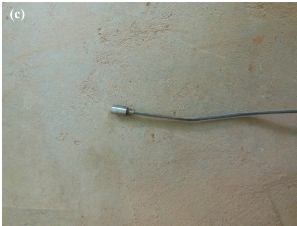
160 Figure 3. Testing instrument equipments . (a) MP-406B sensor of soil Soil moisture sensor (the model is MP-406B) . (b) 161 M-16 collector of soil Soil moisture collector (the model is M-16) . (c) HC-25 m Micro gauge of pore water pressure (the 162 model is HC-25) . (d) MCU collector of pore Pore water pressure collector (the model is MCU) .
