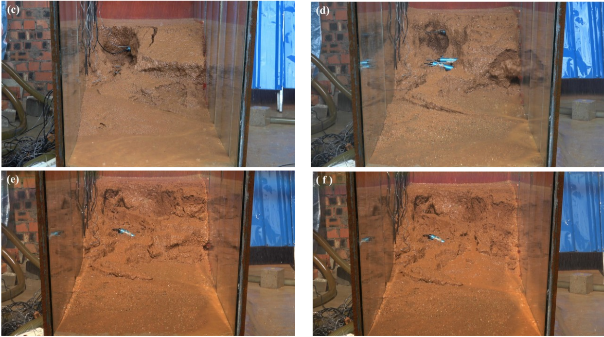
Figure 5. Typical phenomena of test 3. (a) The soil at the slope toe begins to slip after tensile cracks appear. (b) The soil in the middle slope slides. (c) The soil on the slope shoulder slips owing to unbalance internal forces. (d) Blocky soil slides suddenly on the right slope toe. (e) Massive soil on the right slope shoulder slides due to the unloading effect of the slope toe. (f) The slope is stable at the end of the rainfall.
