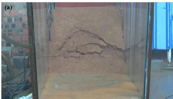
477 478 Figure 20. Typical phenomenon and result with an initial dry density of 1.40 \text{ g cm}^{-3} . (a) Slope failure. (b) Results for 479 sensor #7 closest to sliding surface.
