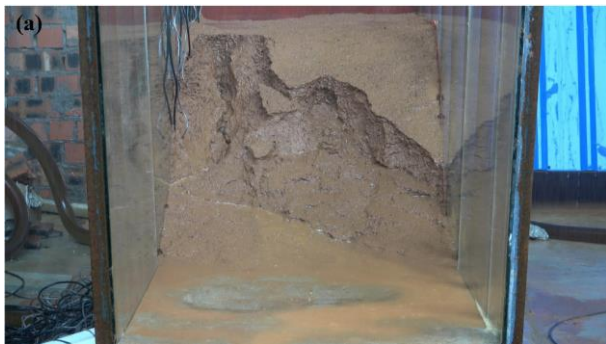
477 478 Figure 20. Typical phenomenon and result with an initial dry density of 1.40 \text{ g cm}^{-3} . (a) Slope failure. (b) Results for 479 sensor #7 closest to sliding surface.
