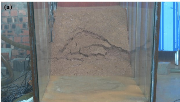
482 483 Figure 21. Typical phenomenon and result with an initial dry density of 1.20 \text{ g cm}^{-3} . (a) Slope failure. (b) Results of 484 sensor #7 closest to sliding surface.
