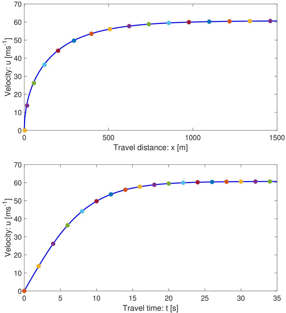
Figure 12: Spatial (top) and temporal (bottom) transportations of the initial velocity ( $u = 0$ ) of the landslide down the slope by the general solution system (39)-(40) as indicated by the star markings for times  $t = 0.0$  s, with 2.0 s increments. These solutions exactly fit with the space and time evolutions of the velocity fields (curves) for the mass point motions given by (8) and (11).
