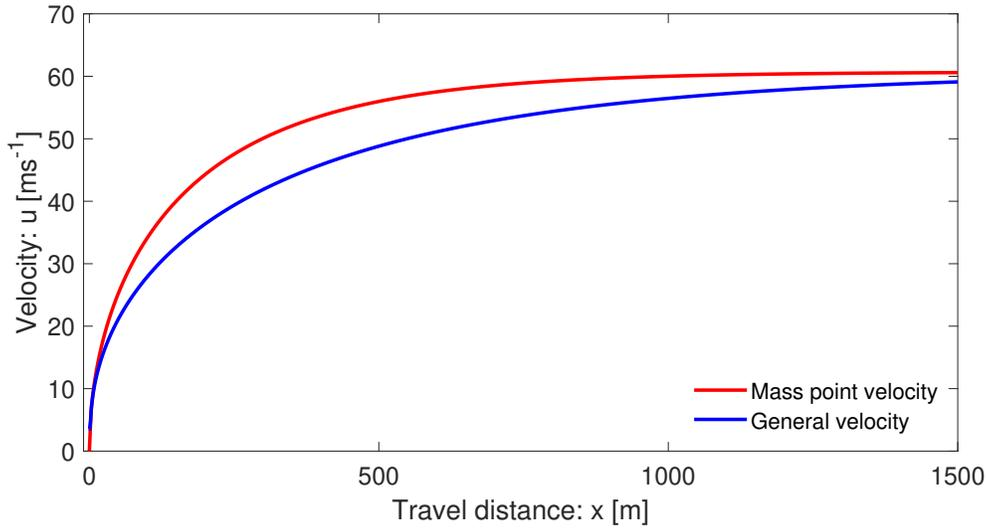
Figure 5: Evolution of the velocity field along the slope as given by (35) for general velocity against the mass point (or, center of mass) velocity corresponding to (8).
