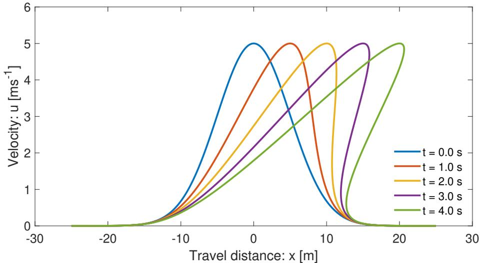
Figure 14: Recovering the Burgers' shock formation and breaking of the wave by the solution system (39)-(40) of the new model (5) in the limit of the vanishing external forcing, i.e.,  $\alpha \rightarrow 0, \beta \rightarrow 0$ .
