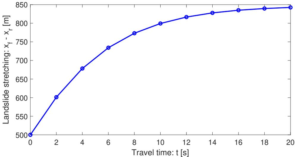
Figure 11: Time stretching of the landslide down the slope including the internal deformation given by the general solution (39)-(40) of (5), corresponding to the initial condition  $s_0(x) = x^{0.65}$  in Fig. 9.
