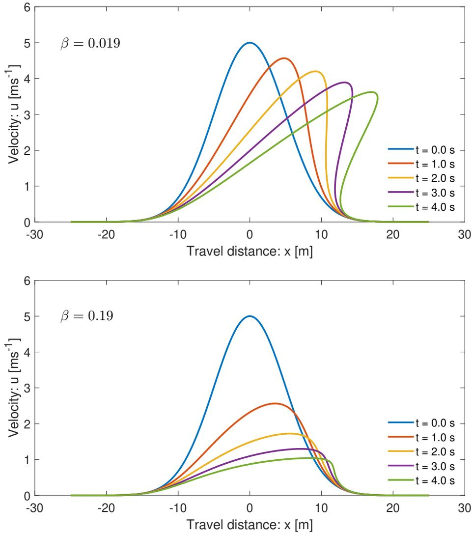
Figure 15: The control of the viscous drag on the dynamics of the landslide. The net driving force is set to zero, i.e.,  $\alpha = 0$ . The viscous drag has been amplified by one and two orders of magnitudes in the top and bottom panels, showing dampened or complete prevention of shock formation and wave breaking, respectively.
