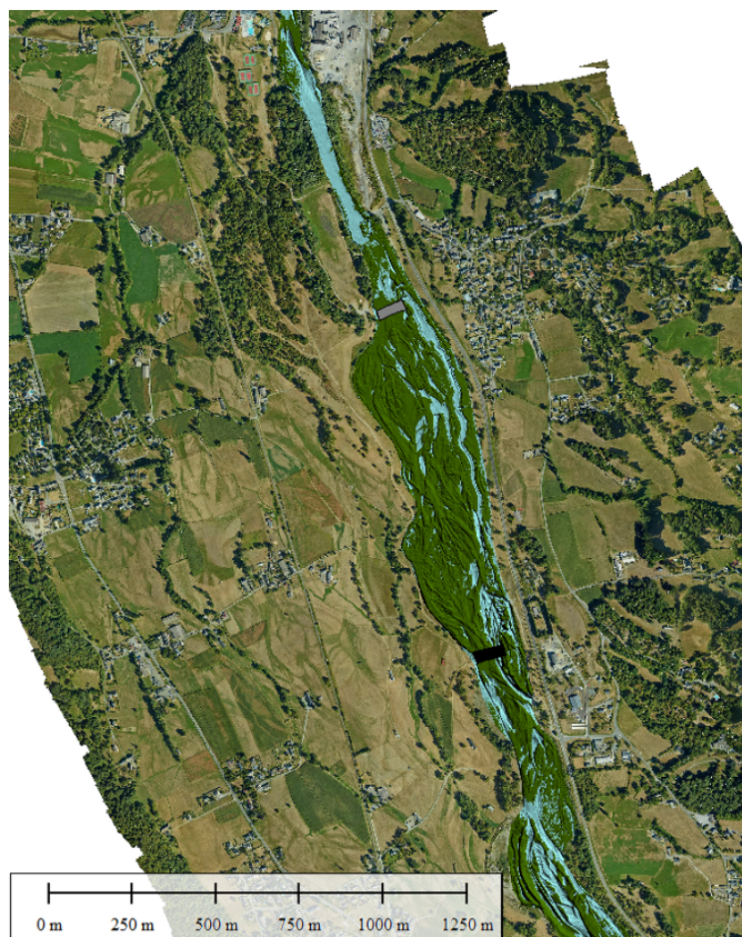
Figure 7. Eroded (light blue) and deposited (dark green) areas in the LDG reach. The upstream weir is represented in black and the downstream weir in grey. This figure illustrates the filling of the LDG as almost all its surface represents deposited materials
