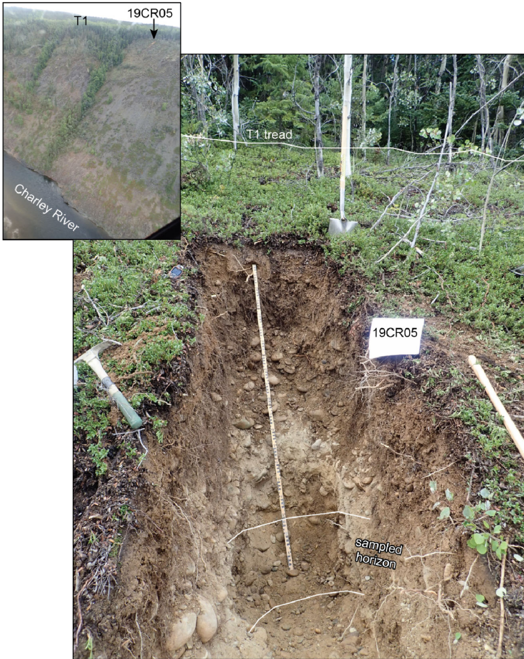
Figure A3. Cosmogenic isochron burial age sample site 19CR05. Site located on Charley River high terrace (T1) in Alaska near the Charley-Yukon River confluence. Inset aerial photo is taken looking southwest; Charley River flow is to the right.
