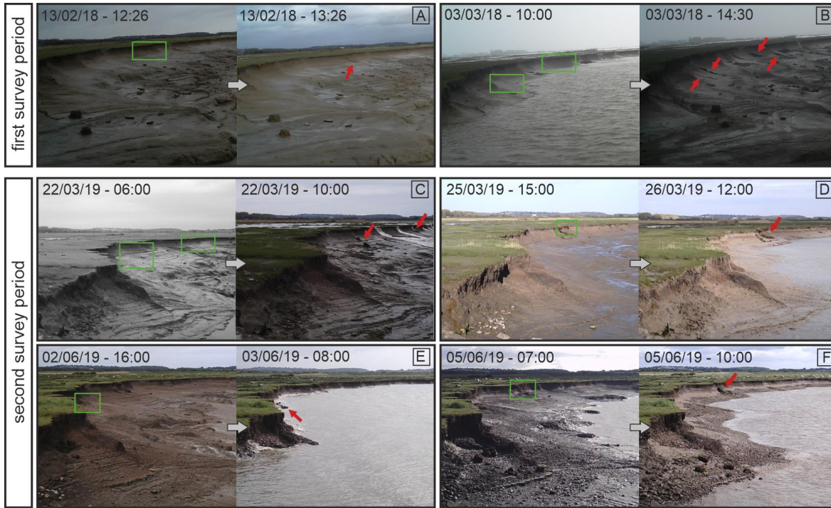
Figure 4. Time sequences of notable mass failure events identified at the study site during the two periods of deployment of the fixed camera. Red arrows in the photographs indicate the collapse events; green boxes highlight the site of the bank where successive collapses occur. Photographs connected by white arrows are successive (very close) in time. The failure events are also highlighted in the tidal range charts in Figure 3.
