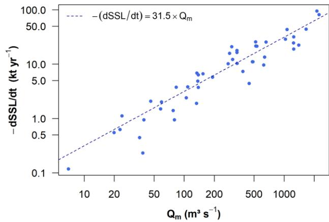
885 **Figure 8:** SSL-decline ( $-\text{dSSL/dt}$ ) as a function of discharge for all stations with a significant change of SSL between 1990 and 2010. **Linear regression**
