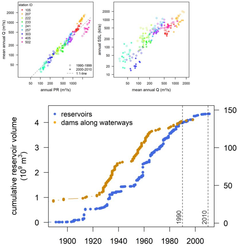
910 **Figure 11: Cumulative volume of reservoirs in Germany and number of dams (barrages) along the German waterways since the start of construction in the 1880ies. The cumulative volume of reservoirs includes only large reservoirs with volumes > 0.04 Mio. m<sup>3</sup> and is taken from Wikipedia ("Liste der Talsperren in Deutschland", accessed at January 2021)**
