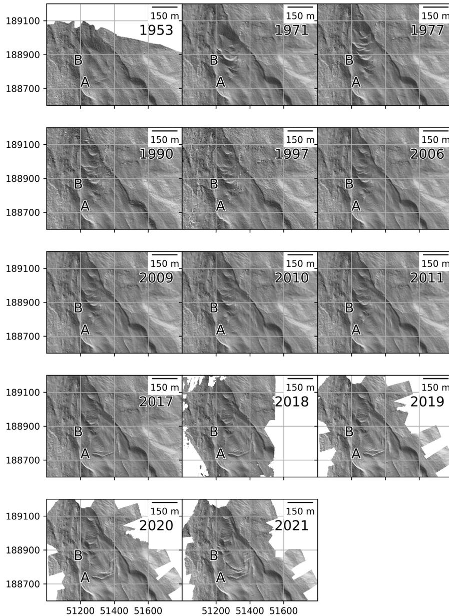
**Figure 7.** Hillshades of DSMs from 1953 to 2021. A and B mark upper and lower sections of morphological destabilization signs as referred to in the text. An animated version of the time series of hillshades is available in the video supplement. (Coordinate grid: EPSG: 31254)
