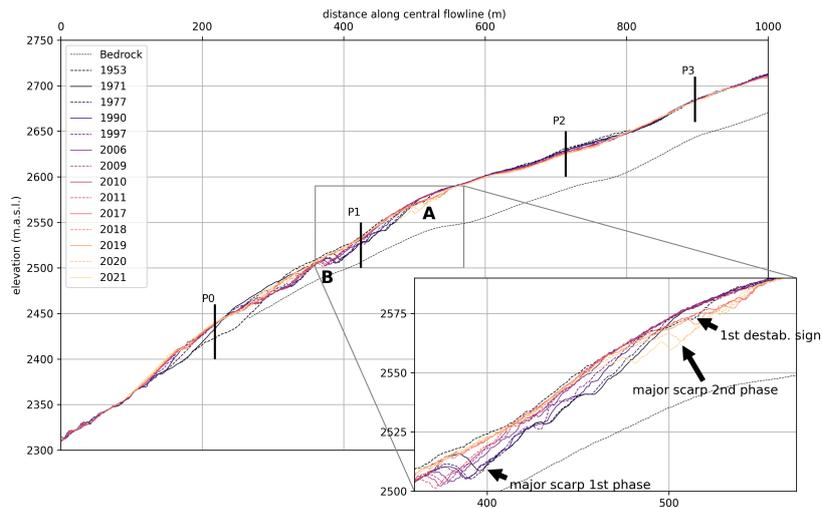
**Figure 8.** Surface elevation along the flow line as extracted from the DSMs. Estimated bedrock profile (dashed line) from Hartl et al. 2016b. Annotations show positions of the cross profiles. A and B mark upper and lower zones of morphological destabilization signs, as in Fig. 7.
