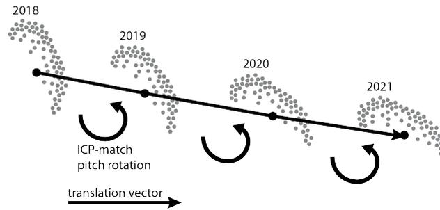
**Figure 4.** Principle of block shape matching in the ULS point clouds (grey dots) between consecutive time steps (2018-2021). The iterative closest point algorithm (ICP) was used to match the shape of a block in one epoch onto its shape in another epoch. A rotation in the opposite direction of the translation can be recognized for the block shapes. The figure shows examples of downslope translation and upslope rotation.
