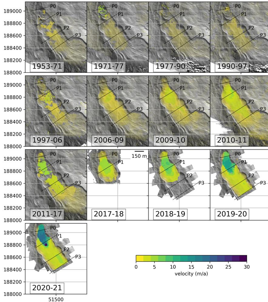
**Figure 6.** Velocity vectors (m/a) for the time series of DSM pairs, plotted over hillshades of the later DSM of each pair. Reference lines defining block profiles P0-P3 added for orientation. (Coordinate grid: EPSG: 31254)
