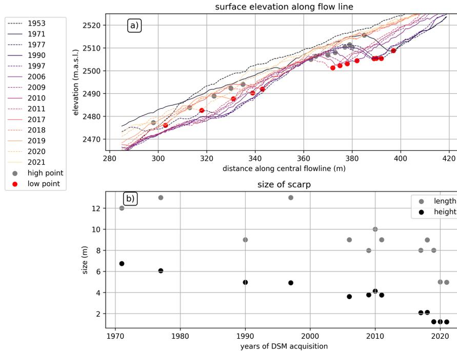
**Figure 10.** a) Surface elevation along the flow line as extracted from the DSMs, zoomed in on the scarp in zone "B", as marked in Fig. 7, and approximate locations of the bottom of the scarp and the high point of the displaced material. The scarp is not yet present in 1953. b) Height and length of the scarp in different years (height is the vertical distance between the respective grey and red dots in a); length is the horizontal distance).
