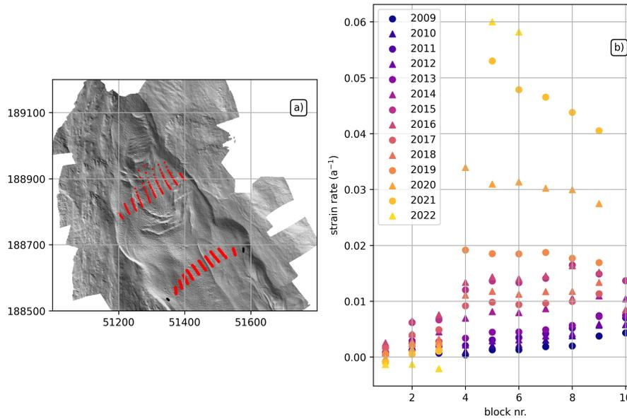
**Figure 12.** Strain rates for the blocks in P1 and P2 (excluding the furthest left and furthest right blocks in P2) for the measurement years 2009/10 to 2021/22. Panel a) shows the location of the blocks in each year (red dots) over the 2021 hillshade. Panel b) shows the strain rate per block pair, counting the blocks in the profile lines from west to east.
